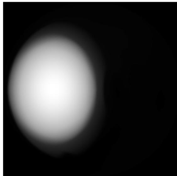
**Figure 5.** *An example photosensor sensitivity fisheye image showing a strong lateral bias. This type of photosensor is often used next to windows to reduce the effect of bright exterior surfaces on the photosensor signal.*
