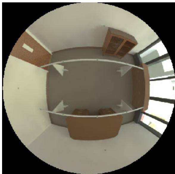
**Figure 4.** *This 180-degree fisheye image shows the model of the room used for validation of the simulation method from the perspective of a photosensor mounted under the pendant luminaire. Notice the windows on the right side showing brightly illuminated exterior surfaces.*
