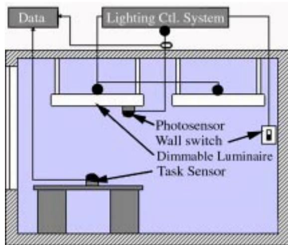
**Figure 1. Schematic diagram of a typical installation of photosensor-based controls in a commercial office. Lines indicate power or data connections between components. Dashed arrows indicate connections and components needed only for collecting performance data.**
