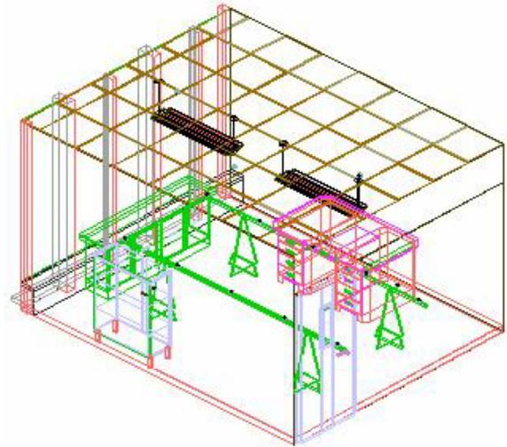
*Figure 8. Wire-line image showing AutoCAD™ 3-D model of the Oakland Federal Building testbed office used for experimental validation of the simulation method.*
