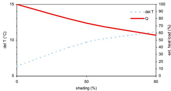
Fig. 6: Temperature gradient and external gains in relation to shading.
