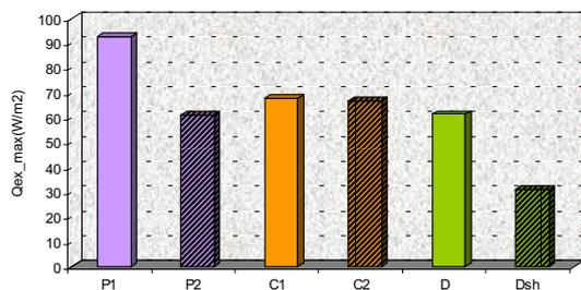
Fig. 2: Max. ext. gains per floor unit area for different facade design variants.
