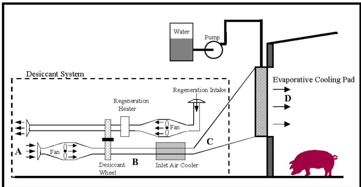
Figure 3. Design concept for swine facility desiccant hybrid system incorporating sensible cooling downstream of the desiccant wheel, followed by further cooling (and humidification) with evaporative cooling.
