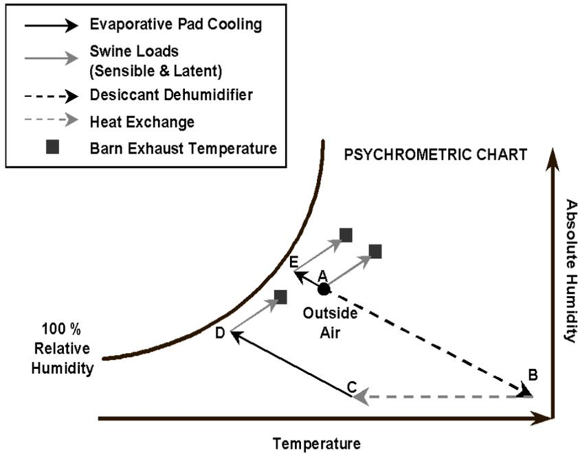
Figure 2. Psychrometric chart plotting the operational conditions for a desiccant-based system using an evaporative pad.
