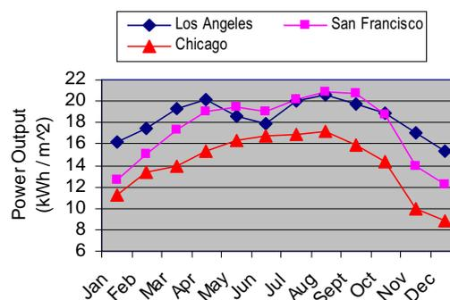
Figure 2: 35 deg. Tilt BIPV Power Output
