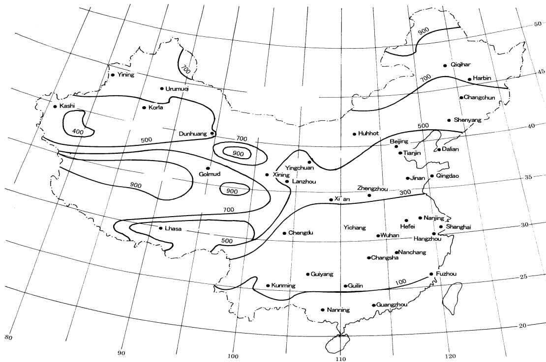
Fig.4 A map with isometric lines of heating loads (The numbers in the figure means the heating loads in \text{MJ/m}^2 )
