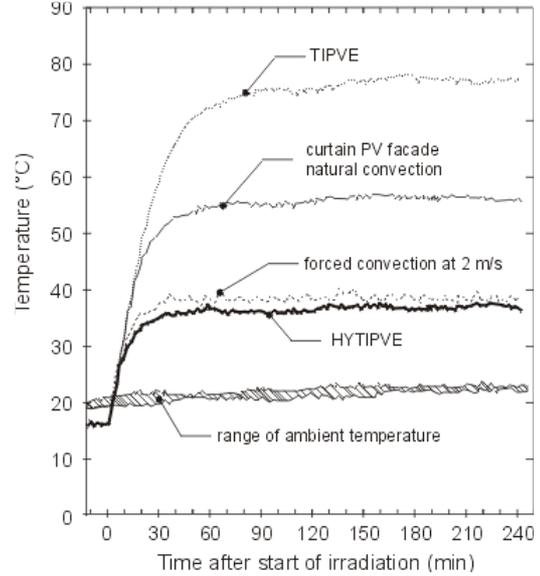
Figure 6. Temperature as a function of time for different types of PV facade elements ( $G=700 \text{ W m}^{-2}$ ).
