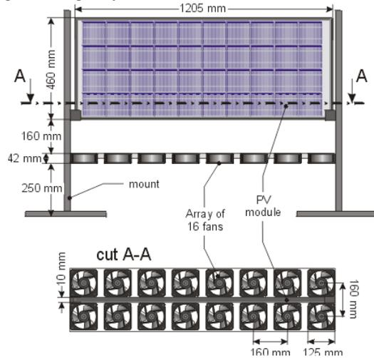
Figure 3. Side- and top view of the actively ventilated PV module.
