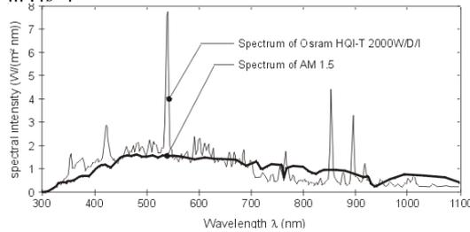
Figure 1. Spectrum of the solar simulator used in the experiments in comparison to AM 1.5.
