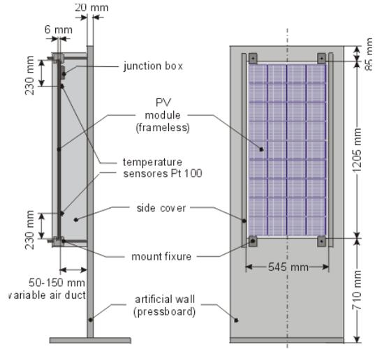
Figure 2. Side- and front view of the passively ventilated PV facade element (curtain facade).
