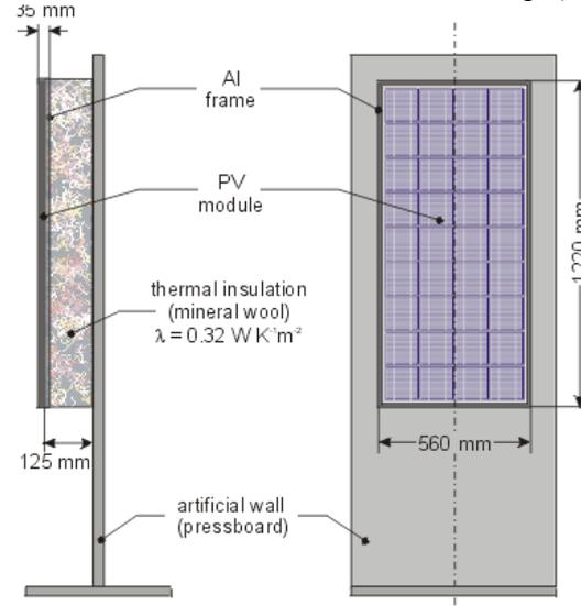
Figure 4. Side- and front view of the thermal insulating PV facade element (TIPVE).
