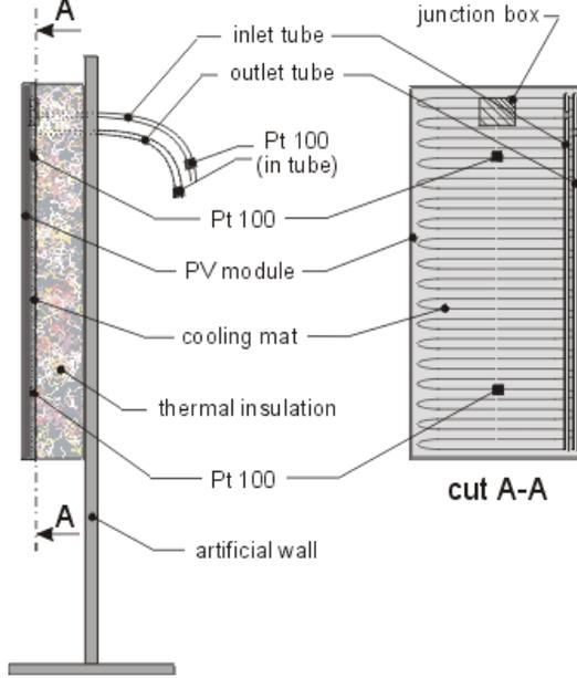
Figure 5. Side- and rear view of the hybrid thermal insulating PV facade element (HYTIPVE).
