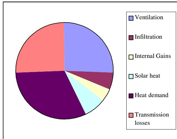
Figure 6: Reference case heat balance (%)
