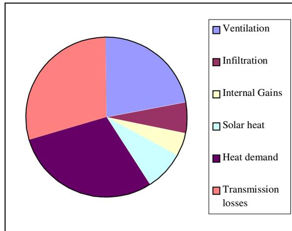
Figure 8: Reduced ventilation case heat balance (%)
