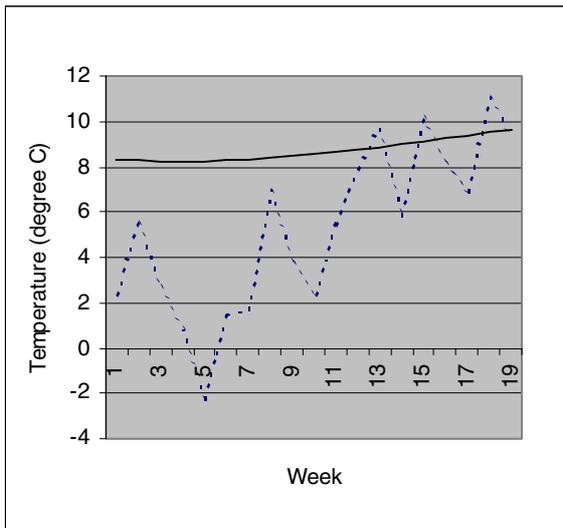
Figure 5: *Temperature beneath ground floor during the first 4 month in wintertime*
