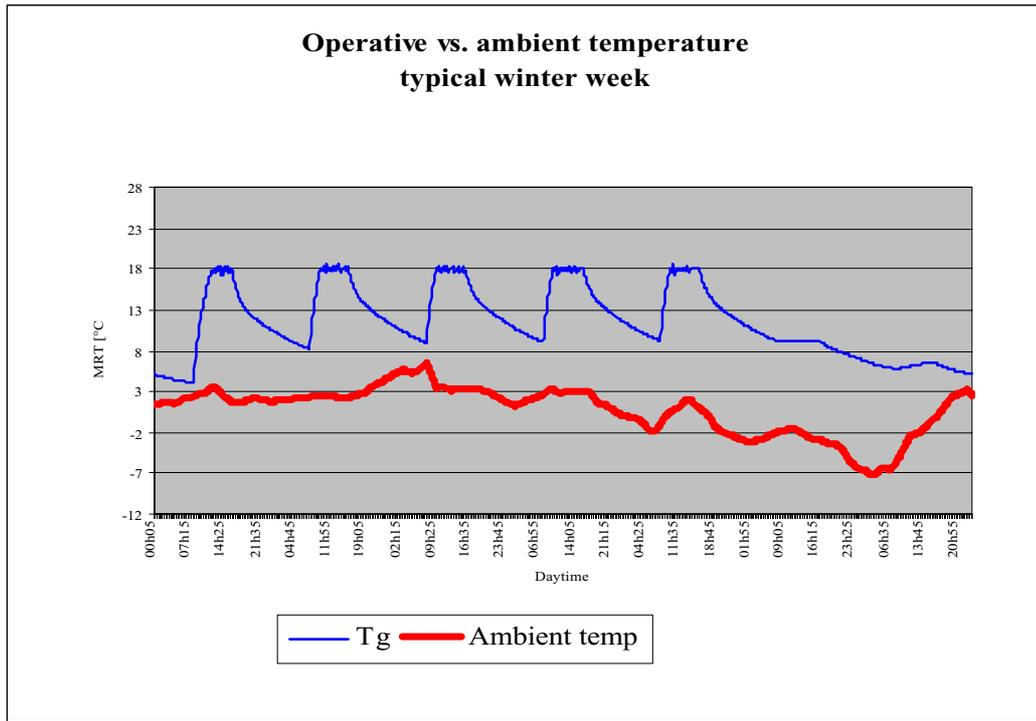
Fig. 6 Operative vs.ambient temperature during typical winter week in the hall with intermittent heating. The hall is heated from 8 AM to 4PM, required temperature is 18°C
