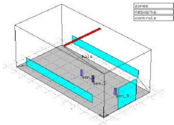
Fig.4 Graphic scheme of the hall with the IR radiant heating. There are 3 sensors, where the MRT was checked, on the ceiling is the IR radiant heater
