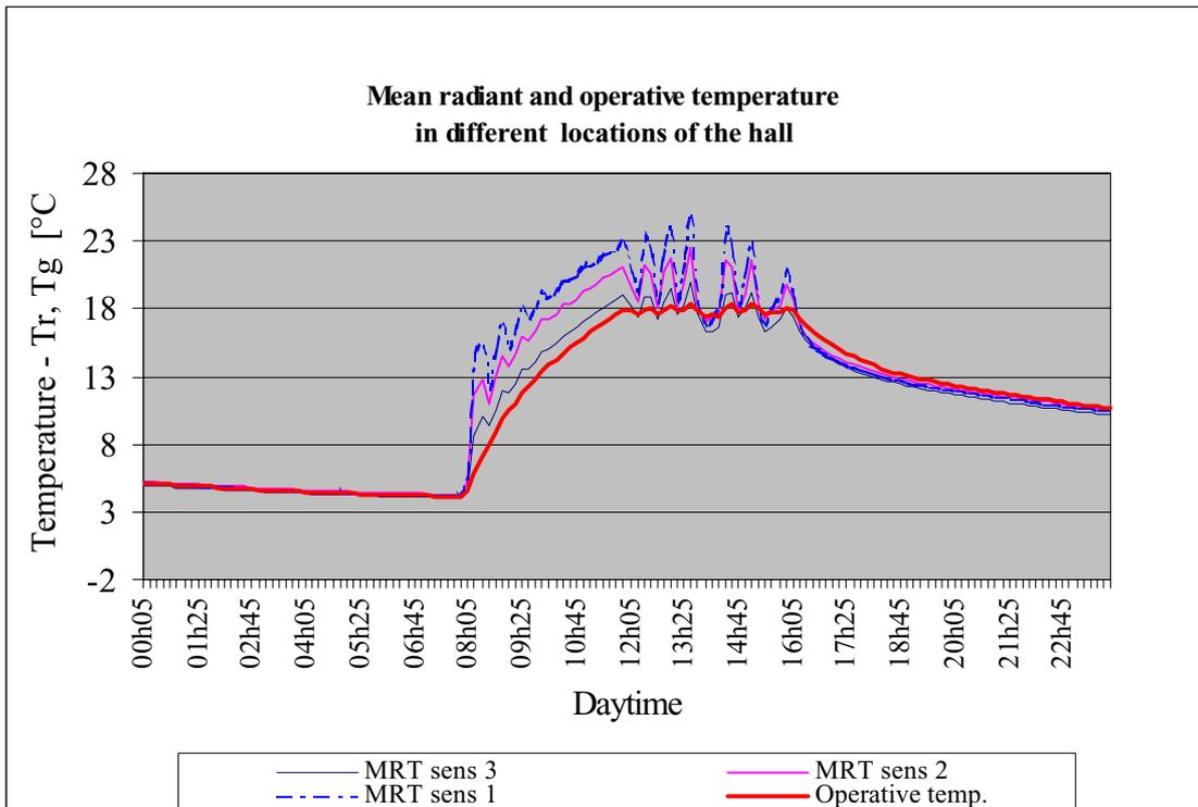
Fig. 7 Mean radiant temepature (MRT) in different locations of the hall during one winter day. Location of the sensors is at the Fig.4
