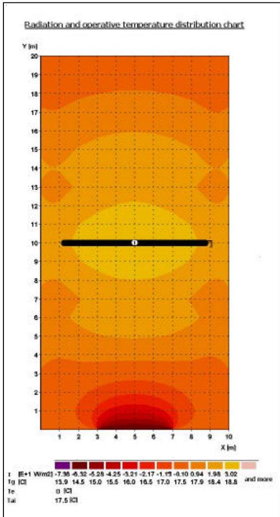
Fig.2 Distribution chart of the operative temperature (Tg) and intensity of radiation (I) on the floor plan of the hall
