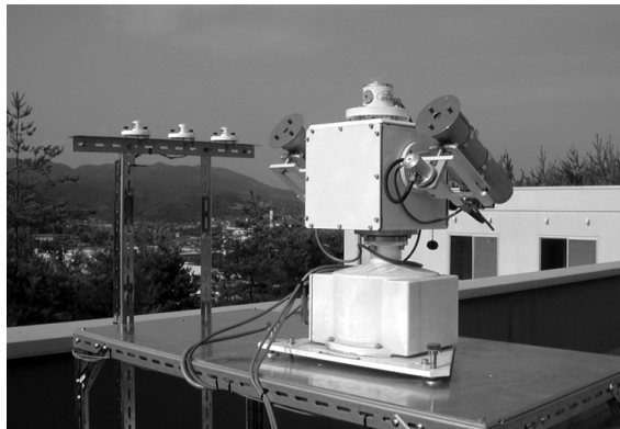
Figure 4 The automated solar tracker, pyranometer and global illuminance meter
