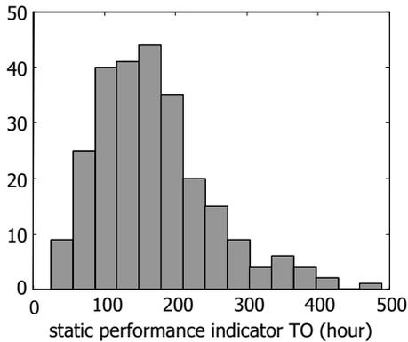
Figure 1 Histogram of the thermal comfort performance indicator, obtained from the propagation of the Latin Hypercube sample of size 250. A common target value for TO is 100 hours.
