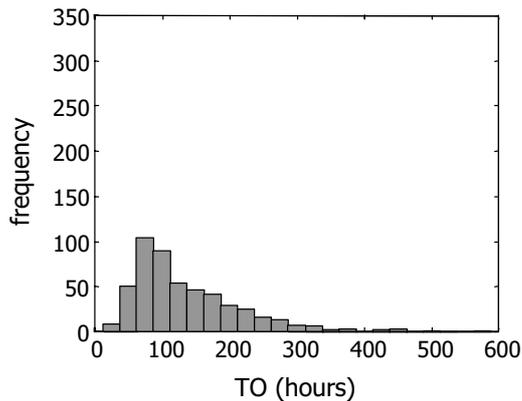
Figure 3 Frequency distributions of the comfort performance indicator TO on the basis of 500 samples. The uncertainty in all parameters is propagated. The left figure shows a histogram of the propagation results, whereas the right figure shows the cumulative relative frequency.
