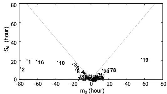
Figure 2 Sample mean  $m_d$  and standard deviation  $S_d$  of the elementary effects on the static comfort performance indicator TO obtained in the parameter screening
