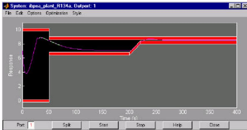
Figure 4: Constraint Envelope – Capacity Command Tracking
