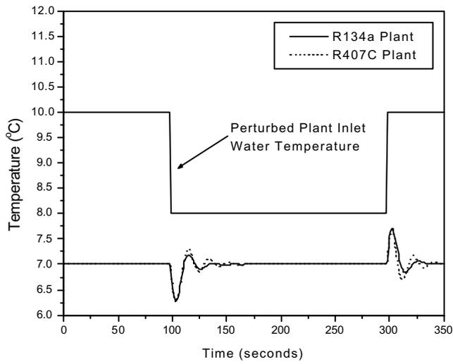
Figure 6: Simulated Load Tracking Response
