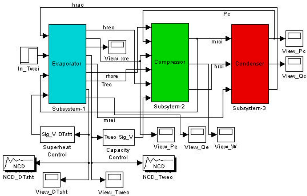
Figure 3: Simulink Model of the Plant
