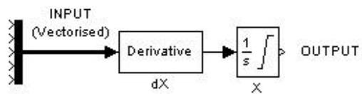
Figure 2: Simulink Template for the Differential Equations
