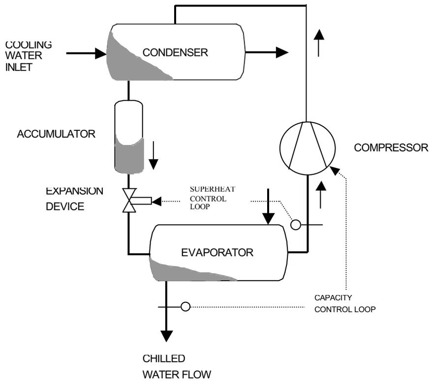
Figure 1: Schematic Layout of the Plant
