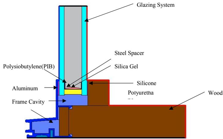
Figure 1. Cross Section of a Window Sill as Installed in Hot Box
