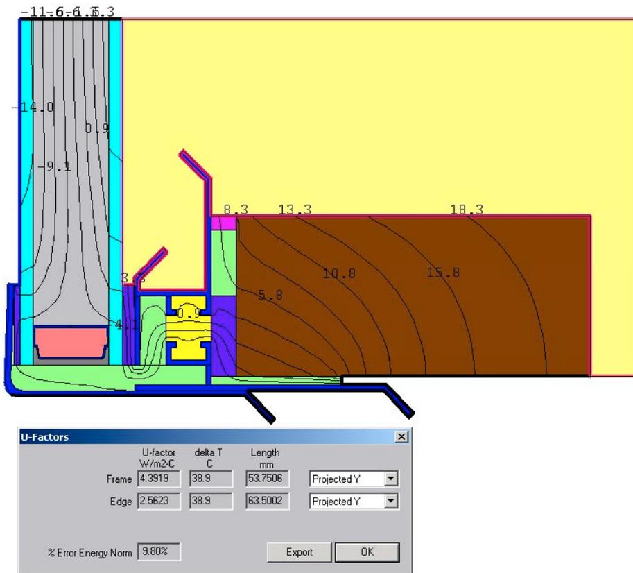
Fig 10 : Isotherms and U-factors for Sill Cross Section in THERM with Radiation Model
