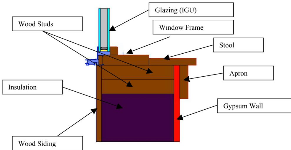
Figure 2. Window in a Typical North American Frame Type Wall
