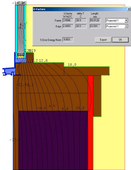
Fig 6: Isotherms and U-factors for Window in a Wall Assembly with Radiation Modeling
