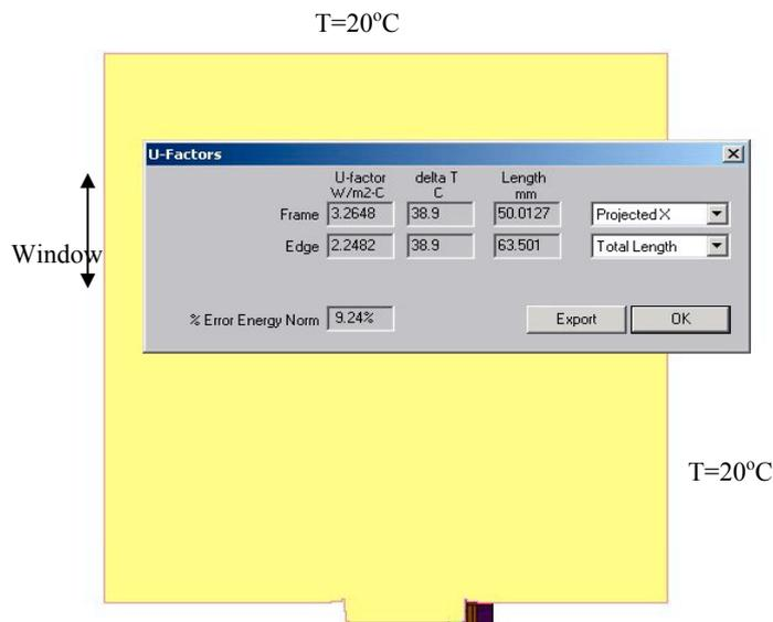
Fig 8: Simulation Model for Window in a Horizontal Position
