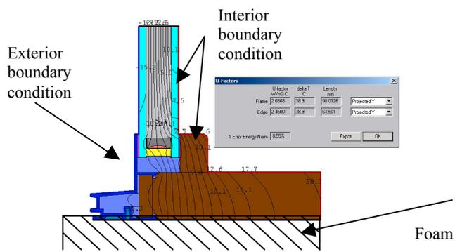
Figure 4. Isotherms and U-factors For The Sill Cross Section
