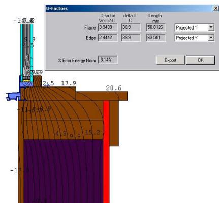
Figure 5. Isotherms and U-Factors for Window Incorporated into Wall Assembly
