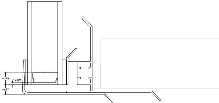
Fig 9 : Typical Cross Section of Skylight
