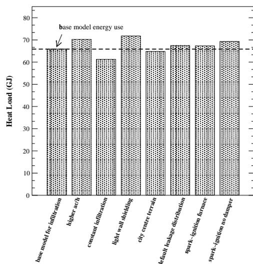
Figure 5: Sensitivity to infiltration factors
