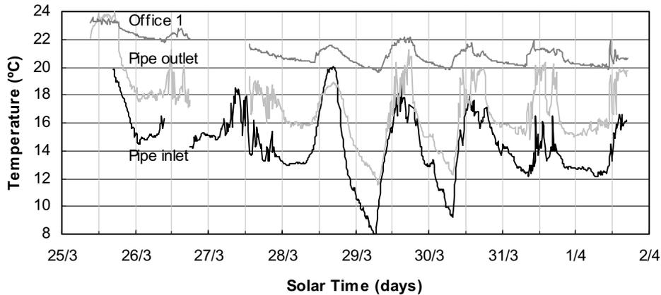
Fig. 8: pipe inlet and outlet temperatures for Office 1.
