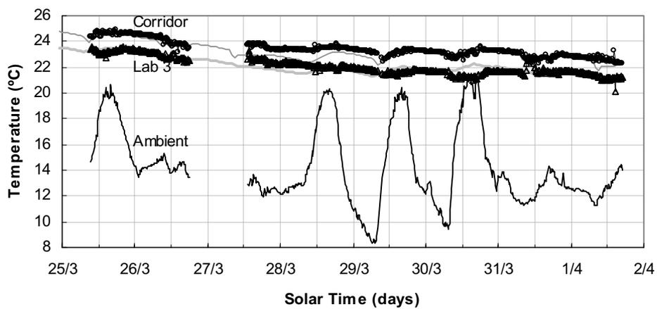
Fig. 7: measured and simulated data for lab 3 and corridor.
