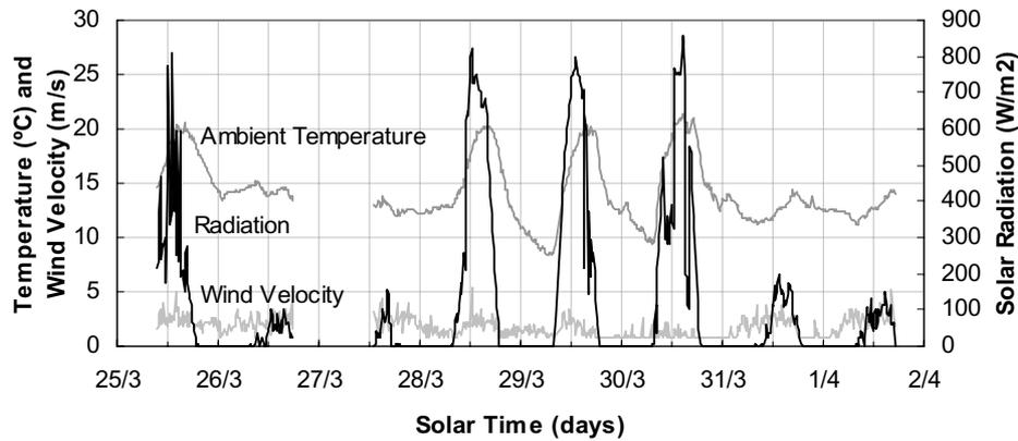
Fig. 3: measured ambient temperature, global solar radiation on a horizontal surface and wind velocity for La Pampa, Argentina.
