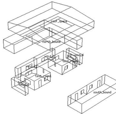
Figure 4: Exploded view of the ESP-r model.
