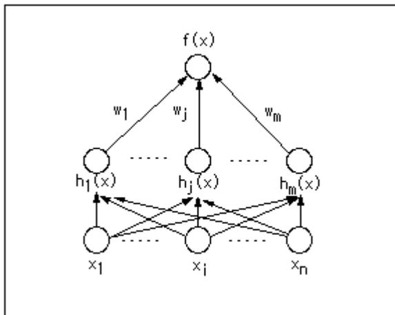
**Fig.02 Radial basis function network**
