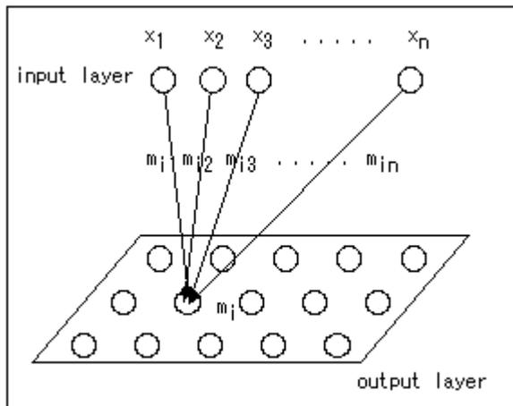
The first layer is the input layer  $x(t)$  of the  $n$  dimension. The second layer is arranged in two dimensions to catch the output visually. The vector that they compete with each other in the second layer is shown in the reference vector  $m_i(t)$ . It has the element of the  $n$  individual in accordance with the dimension of the input layer.
