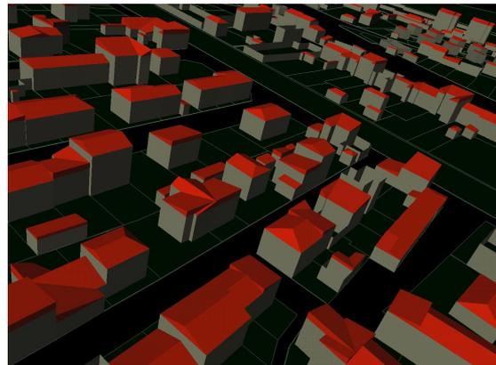
Fig. 2. Automatic 3D reconstruction of a town area.
