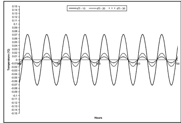
Figure 5: Differences between CLIM2000 results and exact solution for external ( $dTe$ ) and internal surfaces ( $dTi$ )
