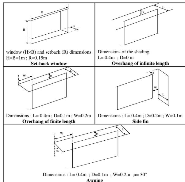
Figure 4: Geometrical description of shading devices
