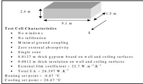
Figure 1: Building characteristics for building level tests
