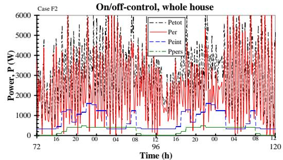
**Diagram 4: Power consumption, on/off-control**
