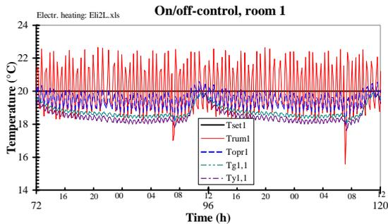
Diagram 6: Temperatures on/off-control, room 1
