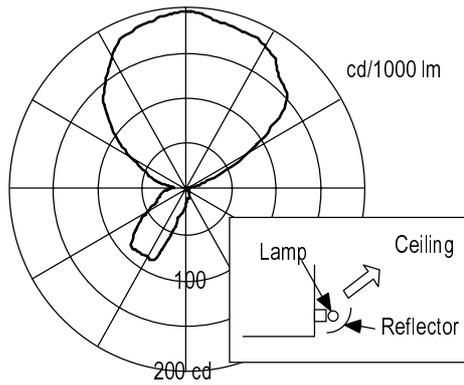
Fig. 6 Luminaire for measurement
