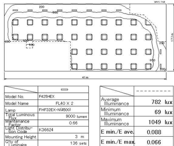
Fig.1 Example of isolux drawing
