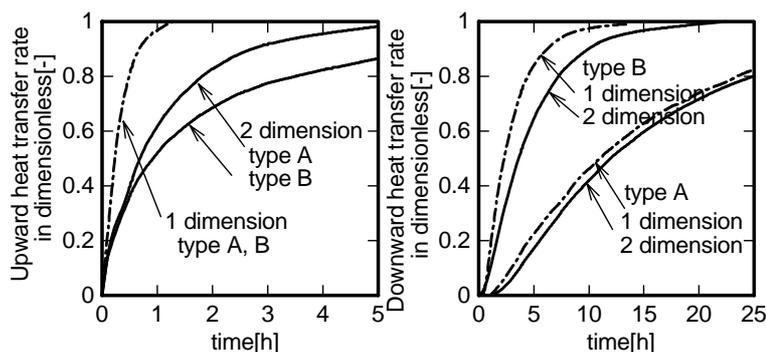
Fig.4 Upward and downward heat transfer rate of standard model
