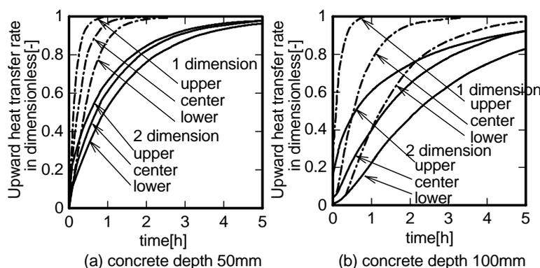
[note] Pipe depth means position of the pipe buried in concrete layer. "upper" and "lower" mean that the distance from upper end or lower end of burying concrete is 12mm respectively.
