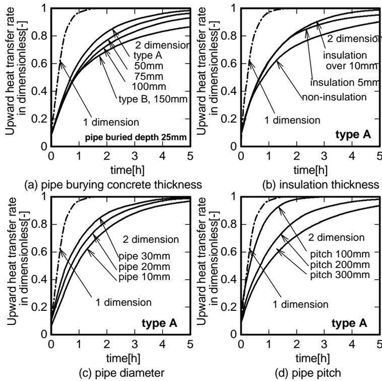
Fig.6 Relationship between major factors and upward heat transfer rate
