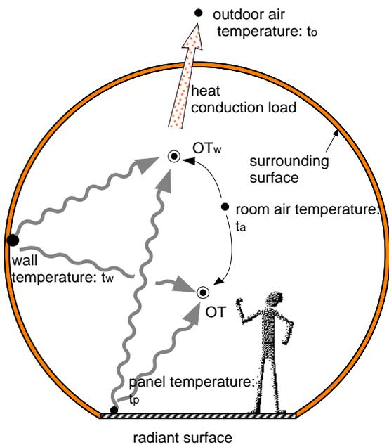
Fig.7 Simplified space comprising radiant panel surface and wall surface
