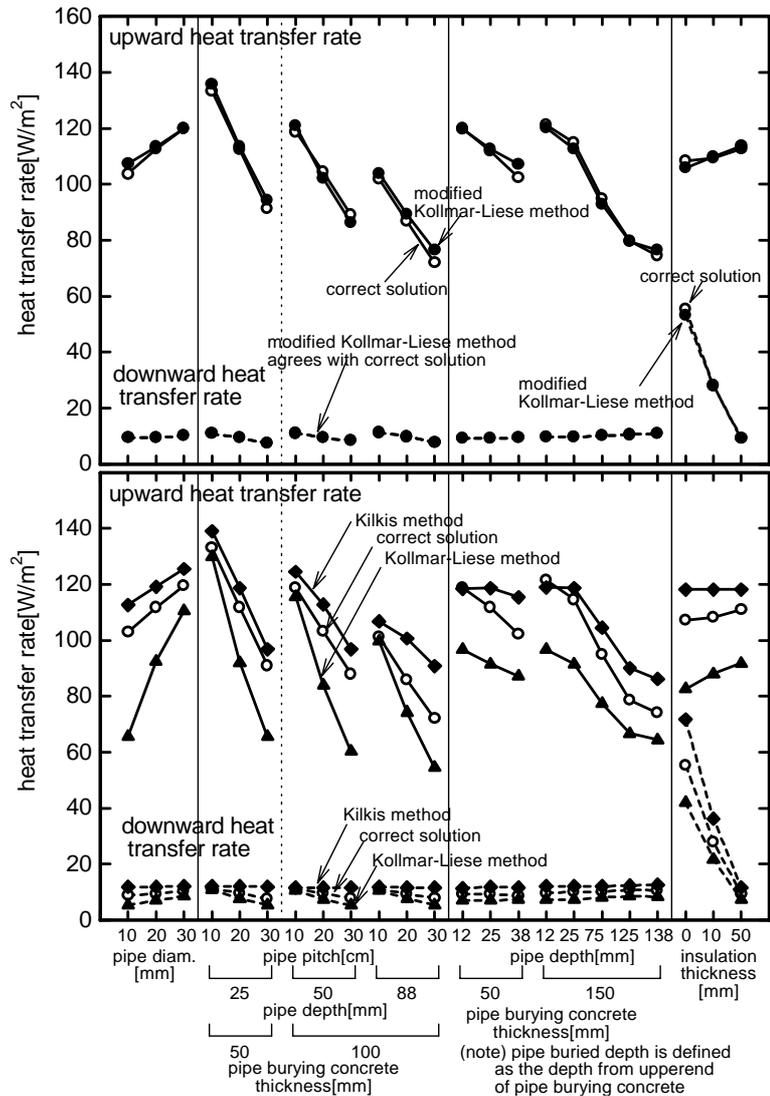
Fig.2 Evaluation of accuracy of modified Kollmar-Liese method and conventional calculation method
