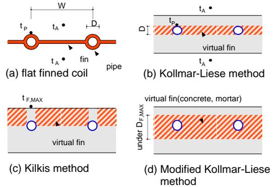
Fig.1 Fin substitution method in each calculation method
