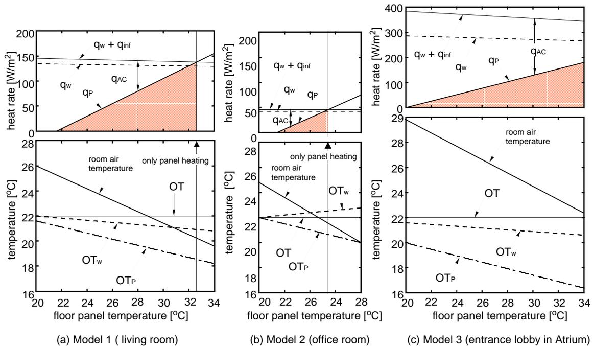
Fig.9 Relationship between floor panel temperature and each of room air temperature, various operative temperatures and heat rate
