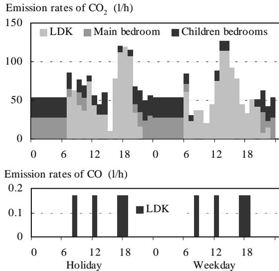
Figure 2 The calculated emission rate of CO<sub>2</sub> and CO
