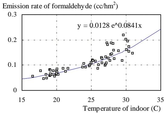
Figure 3 the measured emission rate of formaldehyde in the general detached house constructed in 1995.
