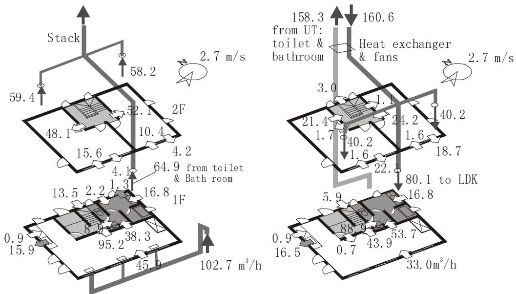
Figure 5 the calculated airflow rates in the house with type-2 and type-3 (the average airflow rates in January )
