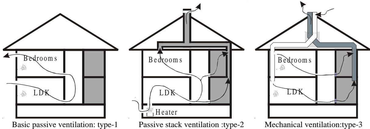
Figure 4 The ventilation systems in the house model
