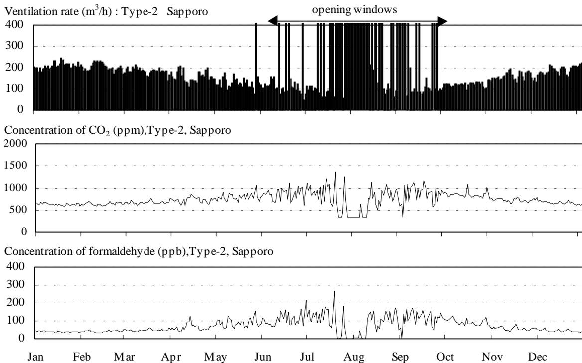
Figure 8 The yearly change of the ventilation rates and the concentrations of the pollutants
