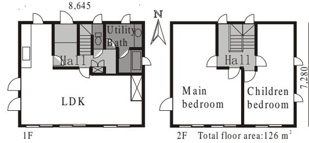
Figure1 The plan of detached house model
