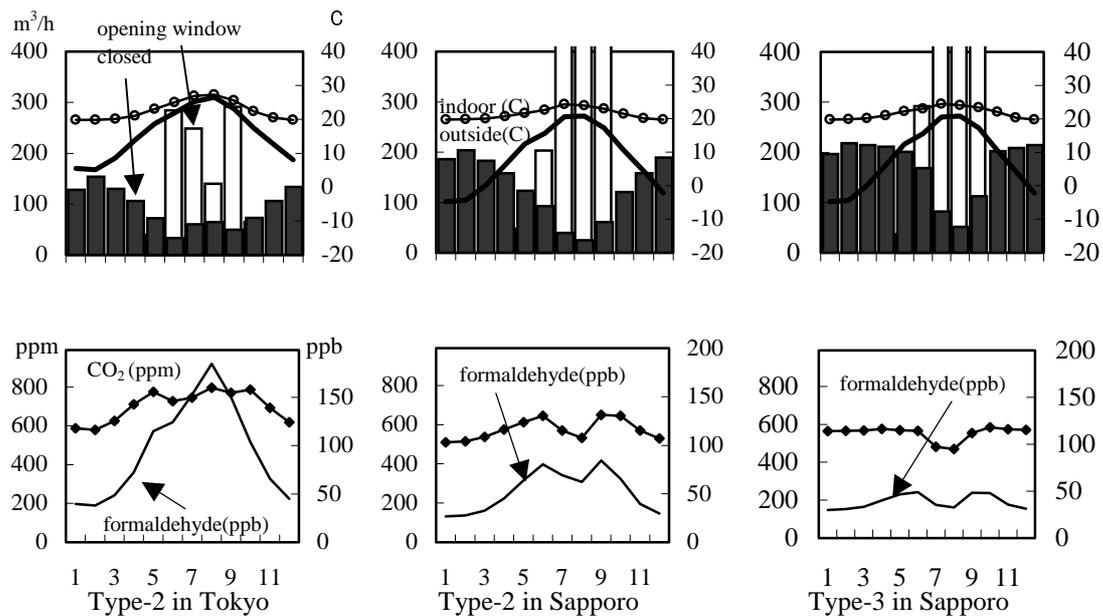
Figure 9 The monthly change of the ventilation rates, the temperatures and the concentrations
