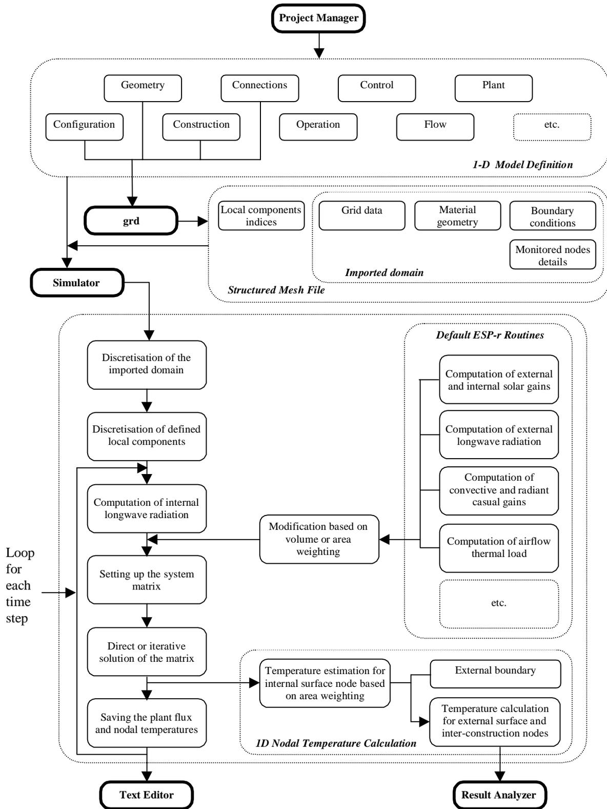
Figure 2. Schematic showing integration of the new module within the ESP-r simulation environment.
