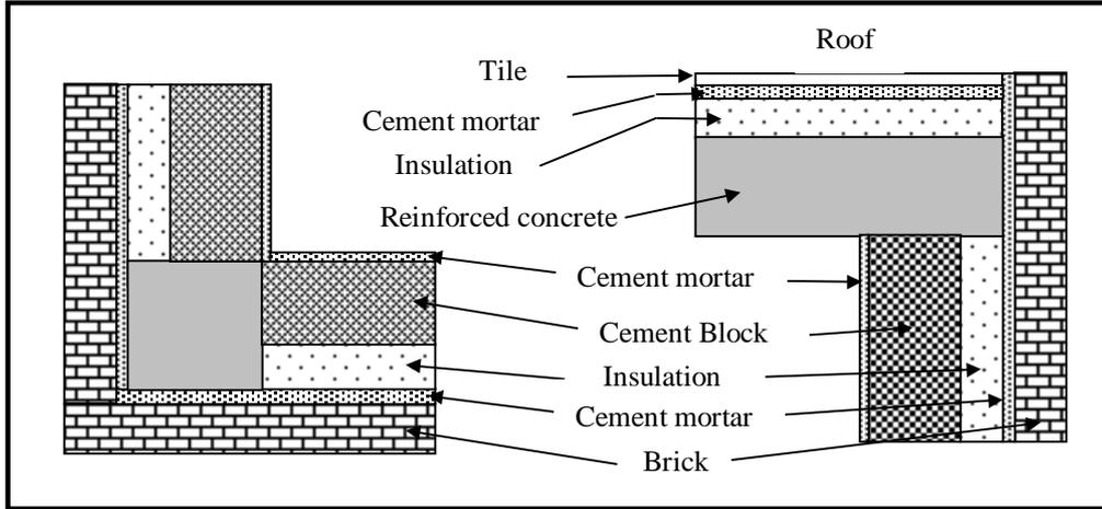
Figure 3: A schematic showing horizontal and vertical cross-sections of a corner
