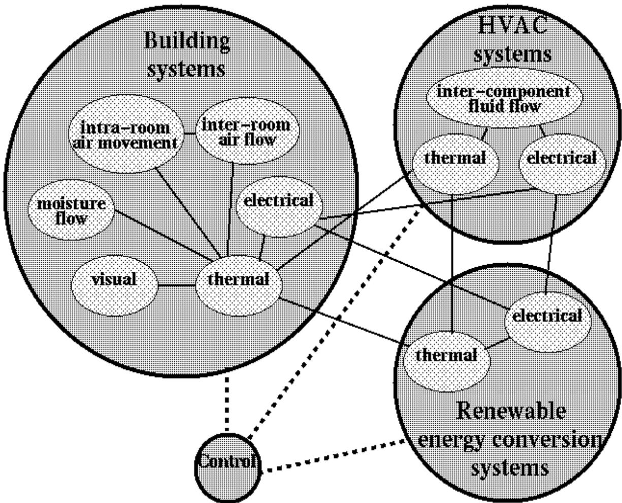
Figure 1: Domain coupling within the ESP-r system.
