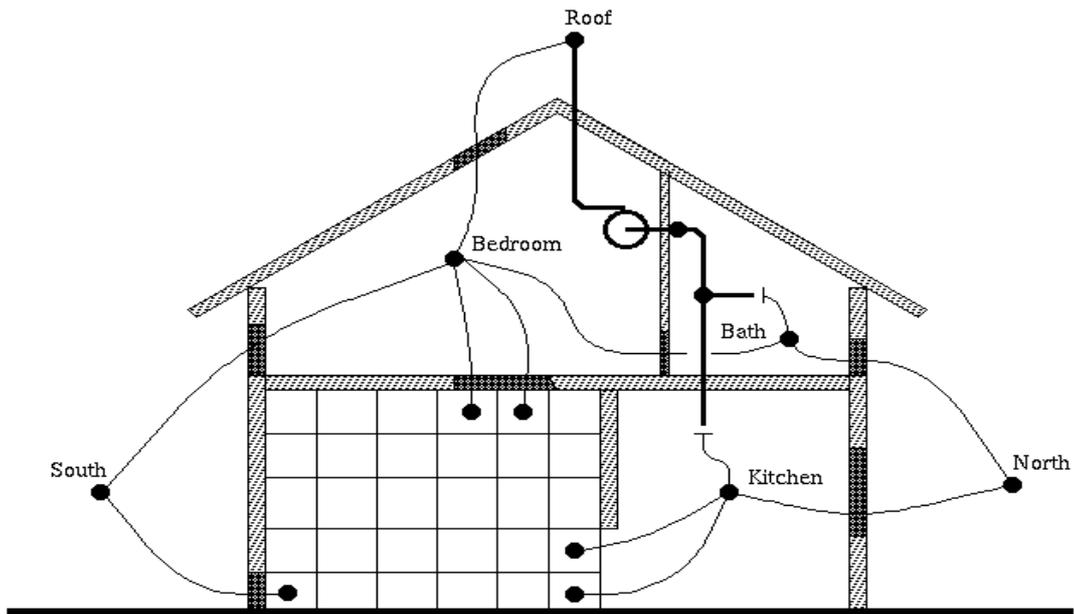
Figure 4: CFD/ network air flow link.
