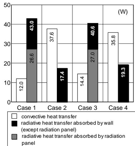
Fig. 8 Characteristics of Heat Transfer from Human Model
