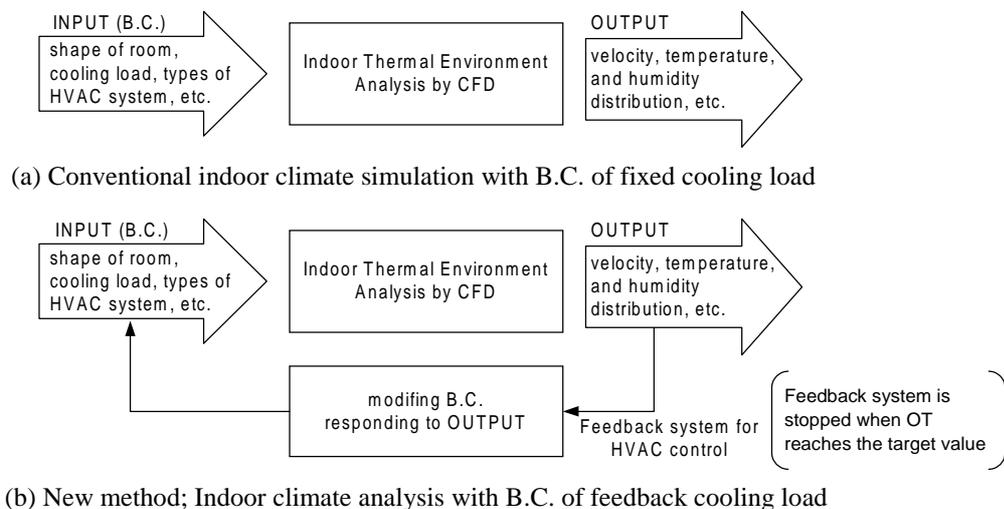
Fig. 1 Concept of Indoor Climate Simulation with/without Feedback System for HVAC Control (B.C. : Boundary Condition, OT: Operative Temperature)
