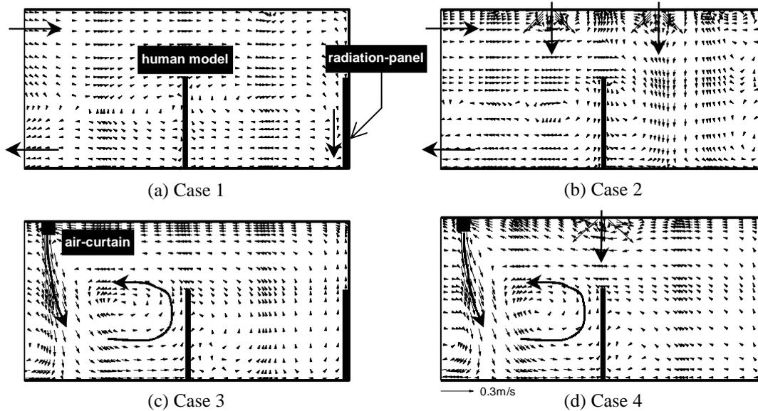
Fig. 4 Flow Fields (Section through center of the room)
