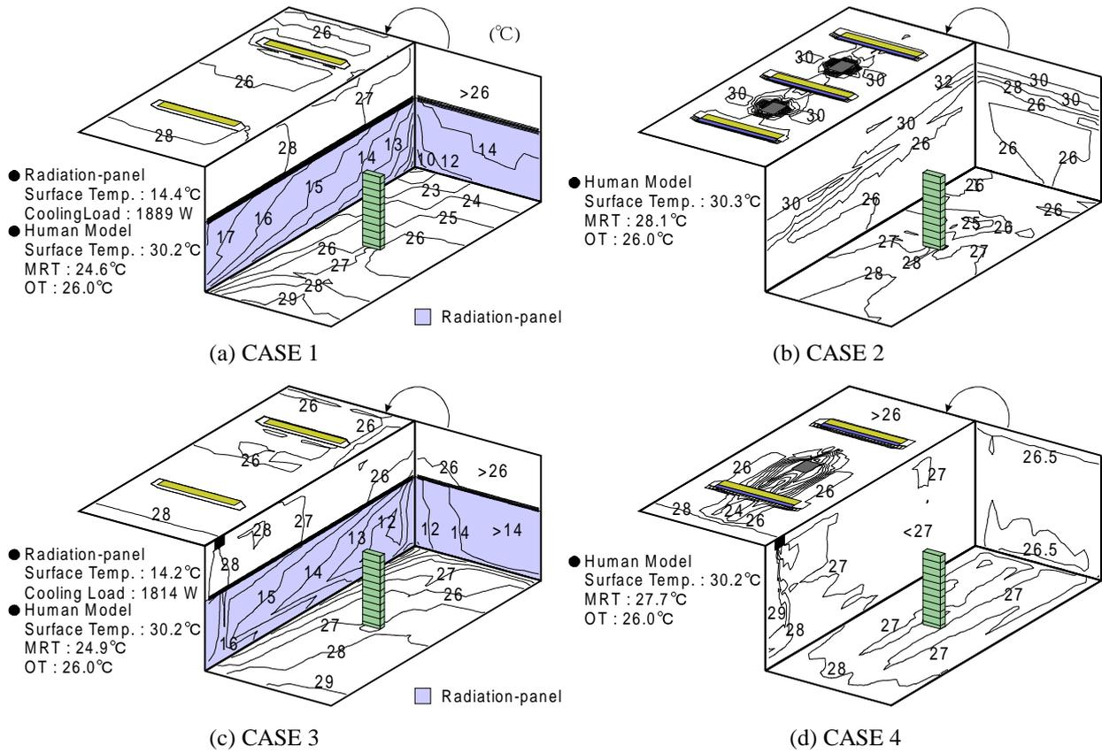
Fig. 7 Wall Temperature Distribution and MRT of Human Model
