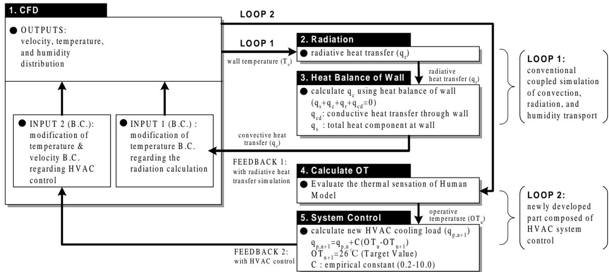
Fig. 2 Procedure of Simulation including HVAC System Control
