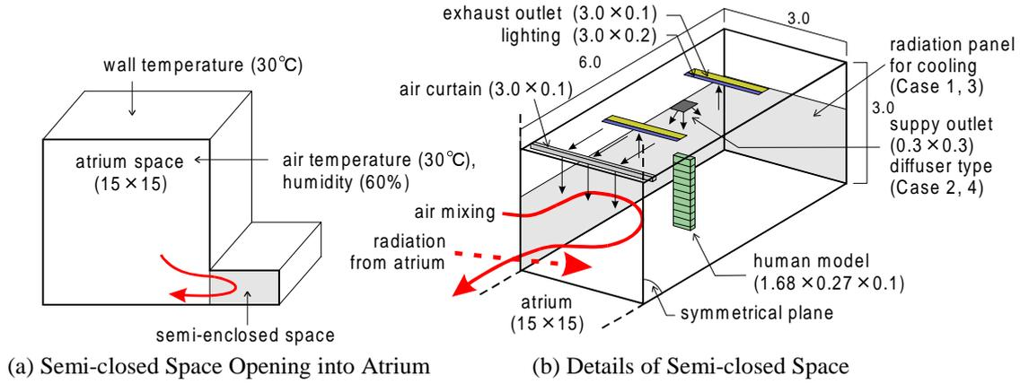
Fig. 3 Semi-enclosed Space for Simulation (unit: m)
