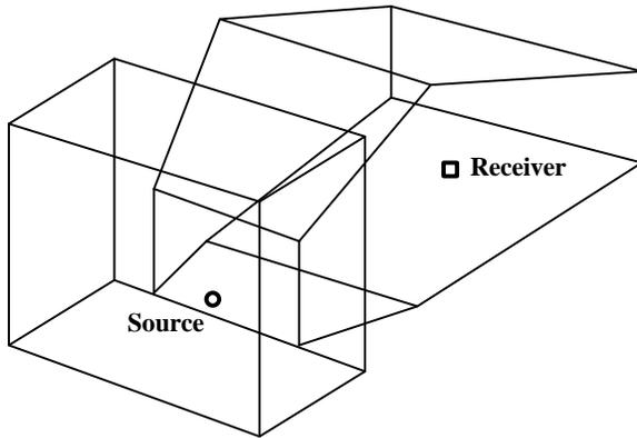
Figure 1. Spatial model of an auditorium showing the enclosing planes. This spatial model is generated by the design system developed by the author.
