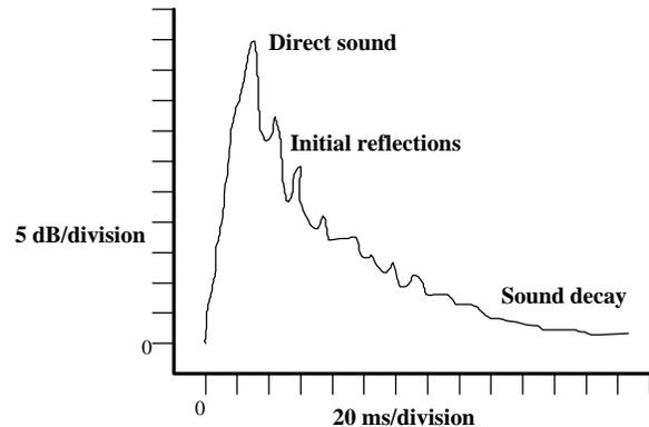
Figure 2. An energy response graph. The intervals shown in the graph are 20 ms (milliseconds). The data in the model is calculated at 1 millisecond intervals.
