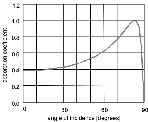
Figure 10: Characteristics of the absorption material that has been applied in the scale model. The diffuse absorption coefficient calculated with Paris’s formula equals 0.56.
