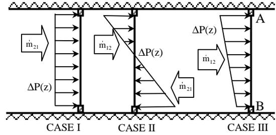
Figure 1. Different configurations of the airflow through large opening
