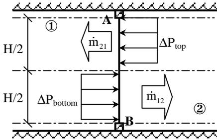
**Figure 2. New model of pressure horizontal gradient in large opening**
