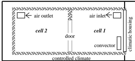
**Figure 3. MINIBAT test cell (Burchiu 1998)**
