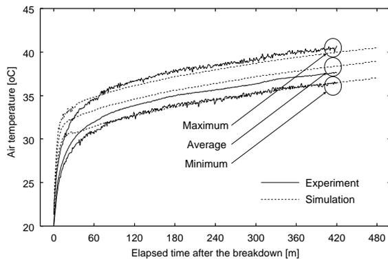
Figure 11: Comparison between experiment and simulation results about room air temperature
