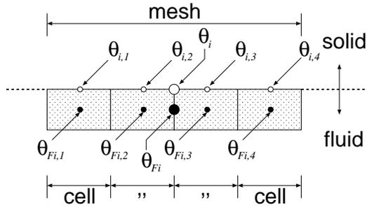
Figure 2: Solid surface mesh and fluid cells
