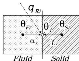
Figure 1: Heat balance at the solid surface
