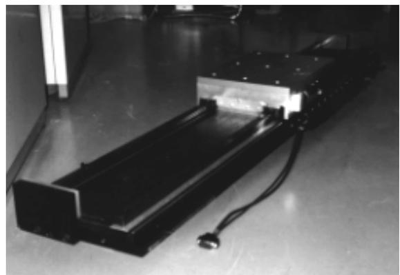
Photograph 1 Thrust motor
