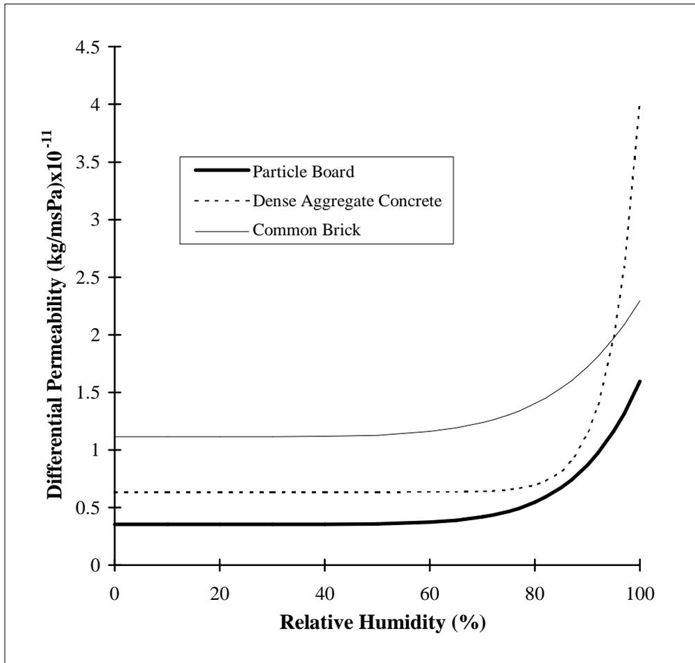
Figure 1 Typical Differential Permeability Curves
