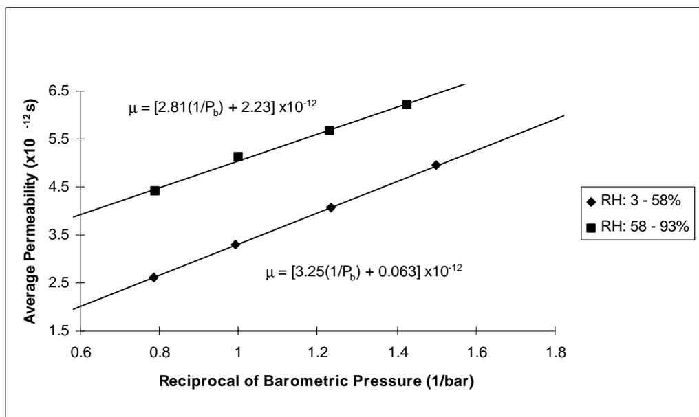
Figure 2 Pressure Test Results for Particle Board
