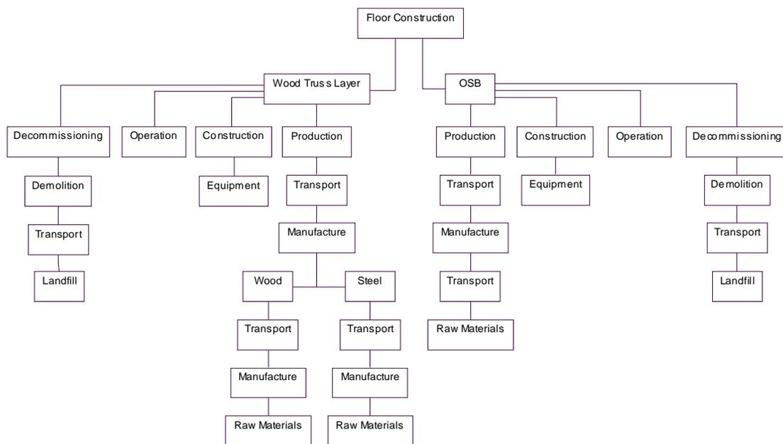
FIGURE 3. Partial representation of a floor construction in ECOLOGUE
