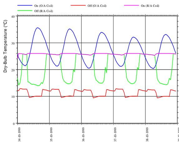
**Figure 4.** Dry-bulb temperature of air entering and leaving the outdoor air and return air coils for the example.
