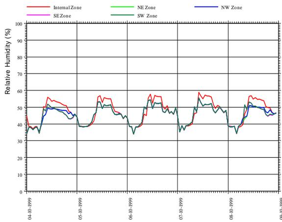
**Figure 2.** Zone conditions for the example with chilled water temperature and flow rate constant throughout the test period.
