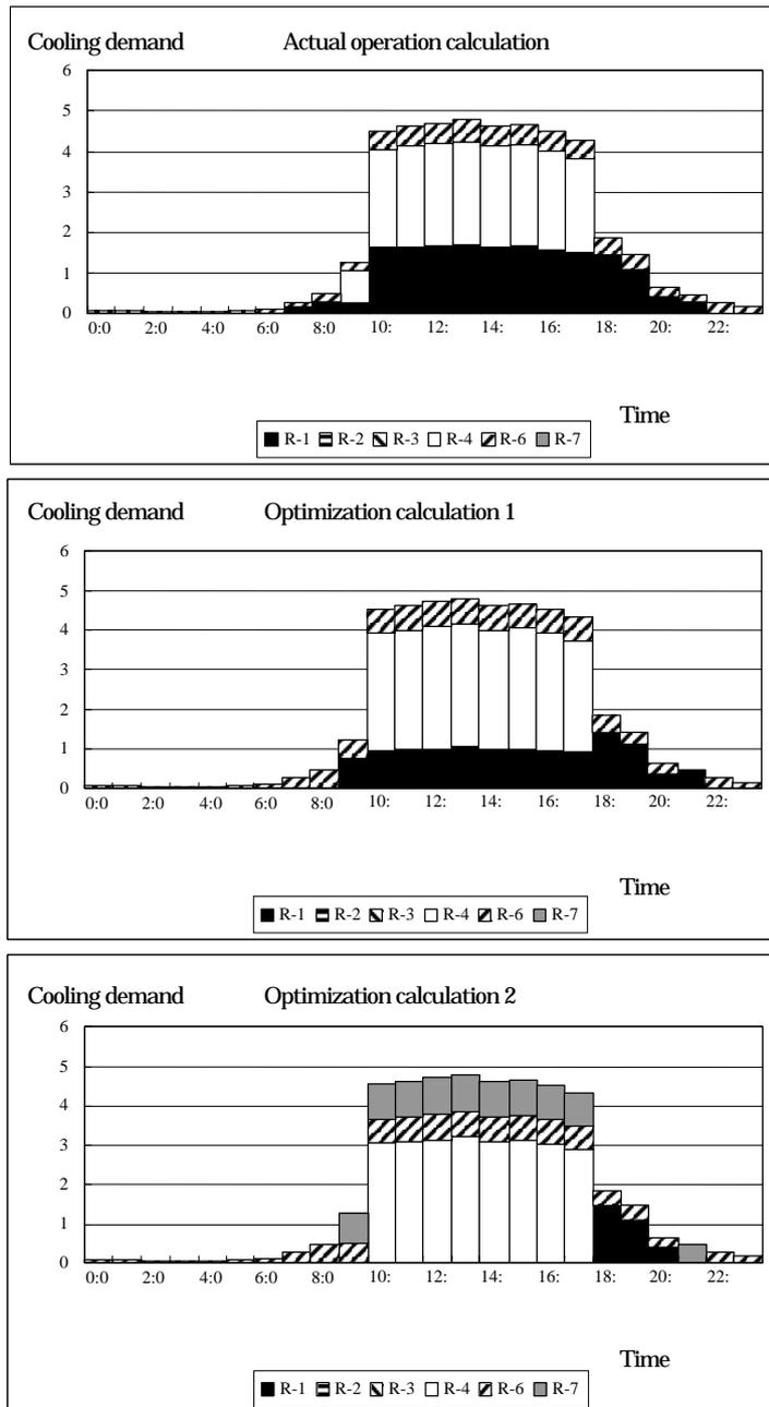
Fig. 9 Heat source operational planning
