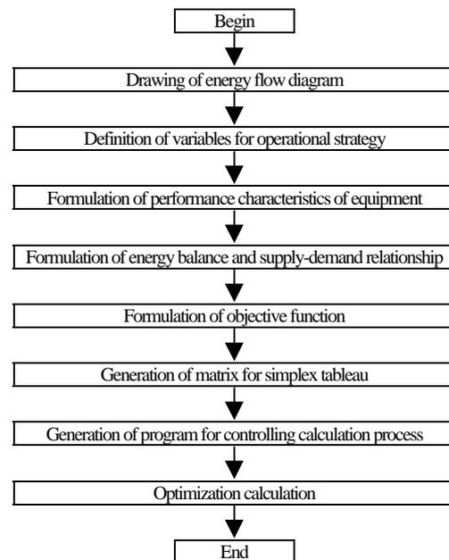
Fig. 1 Procedures of optimal operational planning of energy supply plants
