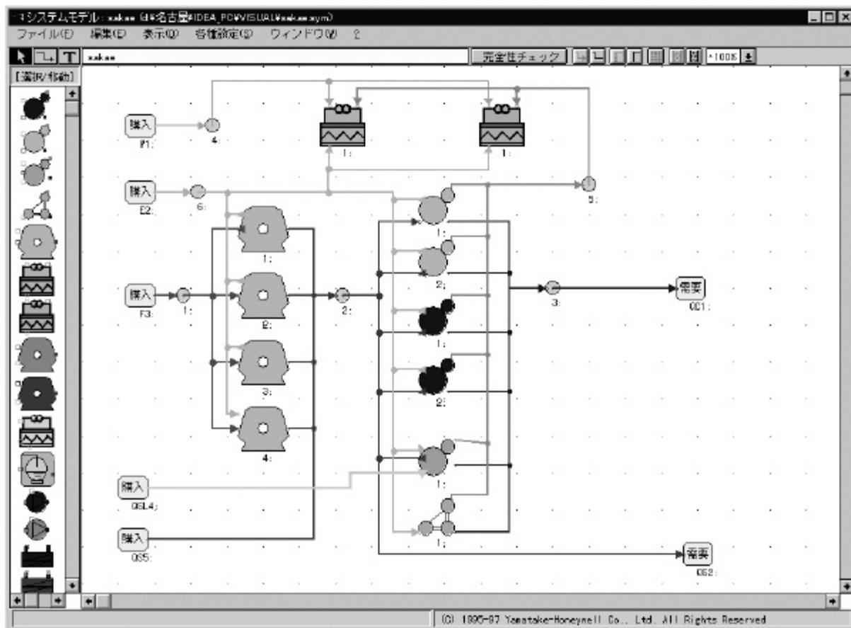
Fig. 6 Example of a plant energy flow diagram drawn by graphical editor
