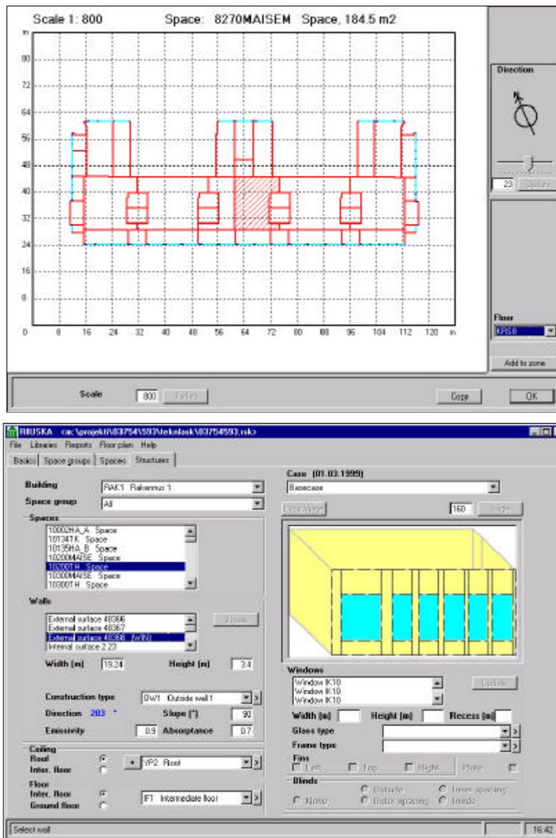
Figure 3 a,b. An example of floor plan and definition of constructions in RIUSKA interface.
