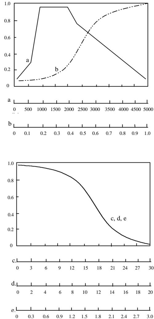
**Figure 3.** Illustrative preference functions for selected performance variable attributes (a: Average illuminance in lx. b: Uniformity c: DGI d: CGI e:  $G_{CRT}$ )
