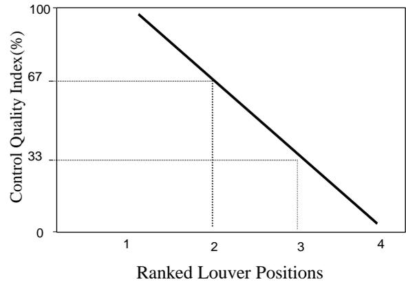
**Figure 2.** Mapping between ranked louver positions and control quality index
