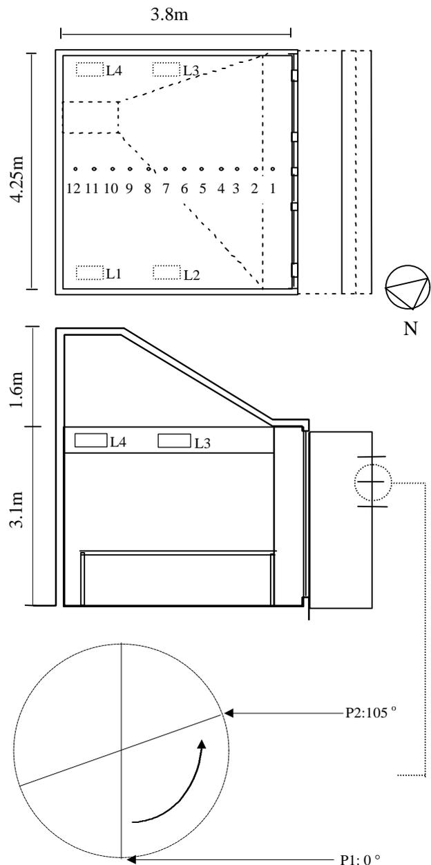
**Figure 1.** Daylight test bed at IW with the sensor, luminaire, and louver arrangement.
