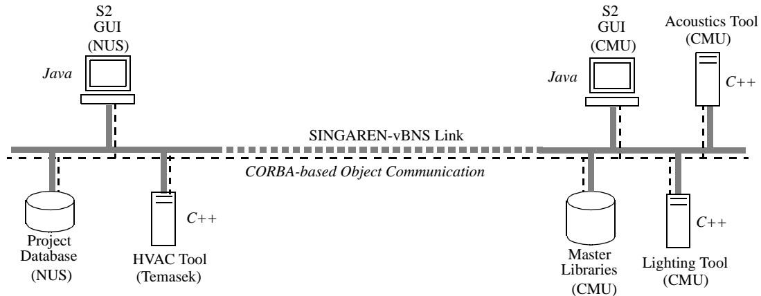
FIGURE 2. Schematic illustration of components of S2 in the case of two distributed users in Singapore and the U.S. collaborating on a building design/engineering project
