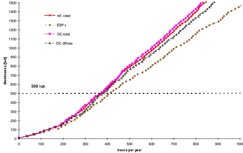
**Figure 4:** The annual cumulative distribution of indoor illuminance levels on the aisle behind the office on the 5<sup>th</sup> floor of the office building
