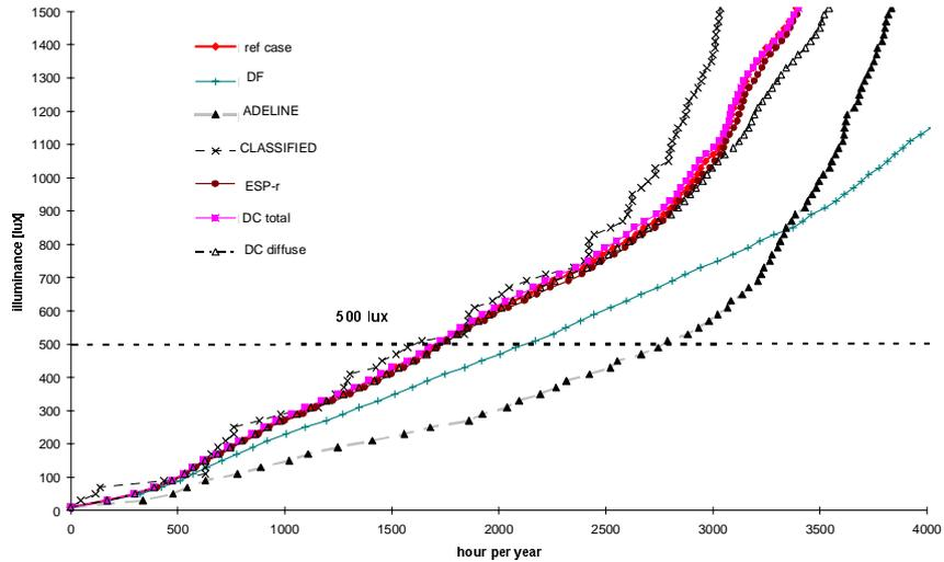
**Figure 3:** The annual cumulative distribution of indoor illuminance levels for a point 2.7 m away from the facade
