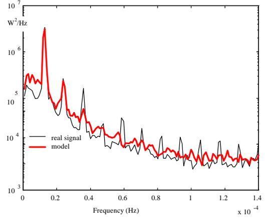
Figure 2. Power spectral density of hourly series of solar flux: estimated from the data and calculated from the model.
