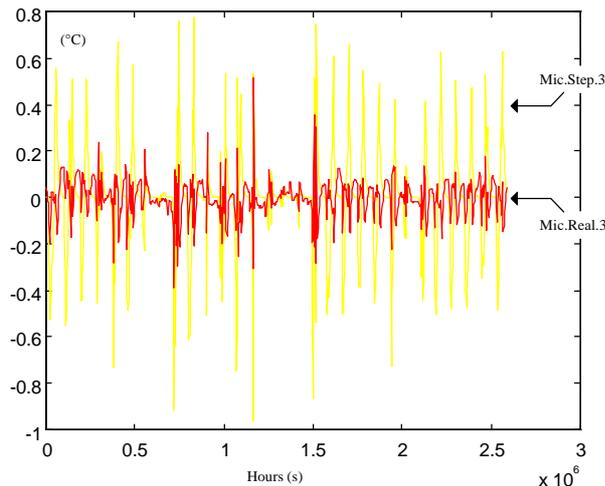
Fig.9.3rd order Michalelesco reduced models (step functions and actual data as inputs).
