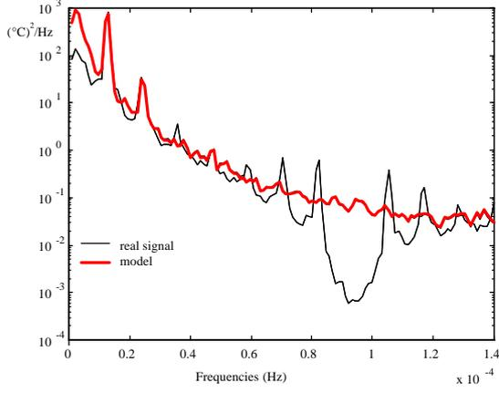
Figure 1. Power spectral density of series of hourly temperature: estimated from the data and calculated from the model.
