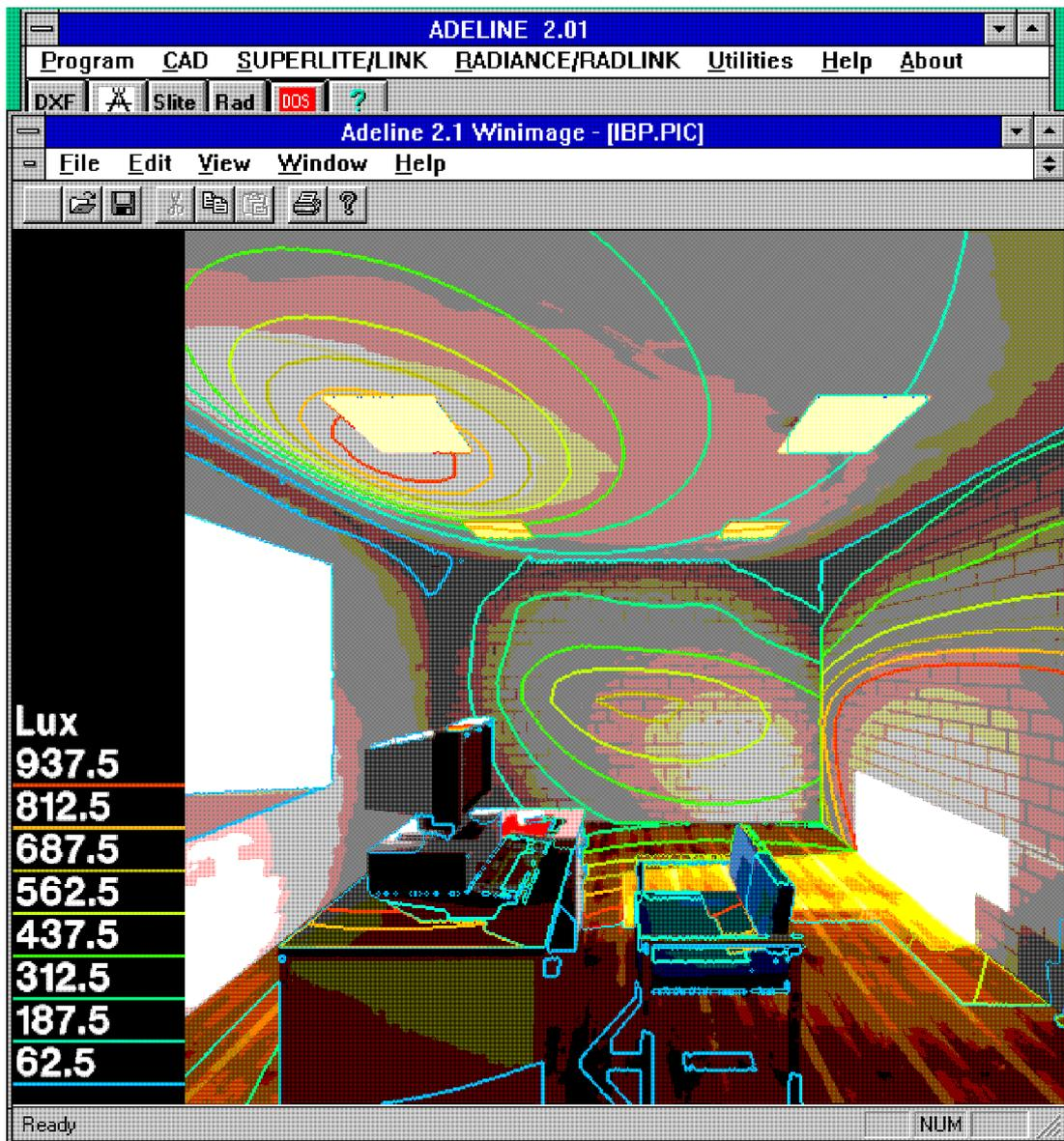
Figure 2: ADELIN graphical user interface under Windows NT. The image background shows the ADELIN main menu, the front shows a photorealistic visualisation generated with RADIANCE NT, displayed from within the ADELIN GUI.
