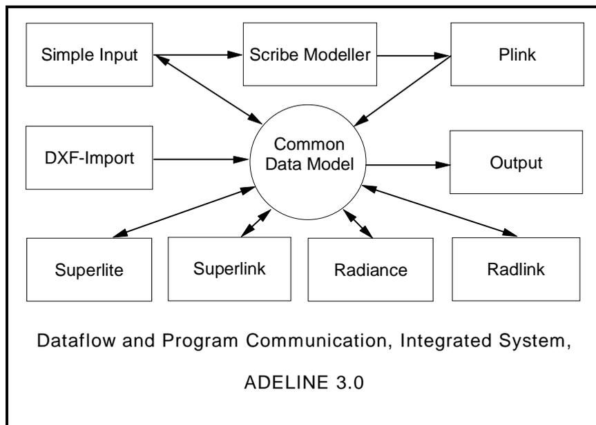
Figure 4: Graphic showing the integration of the different program modules with the common data model.
