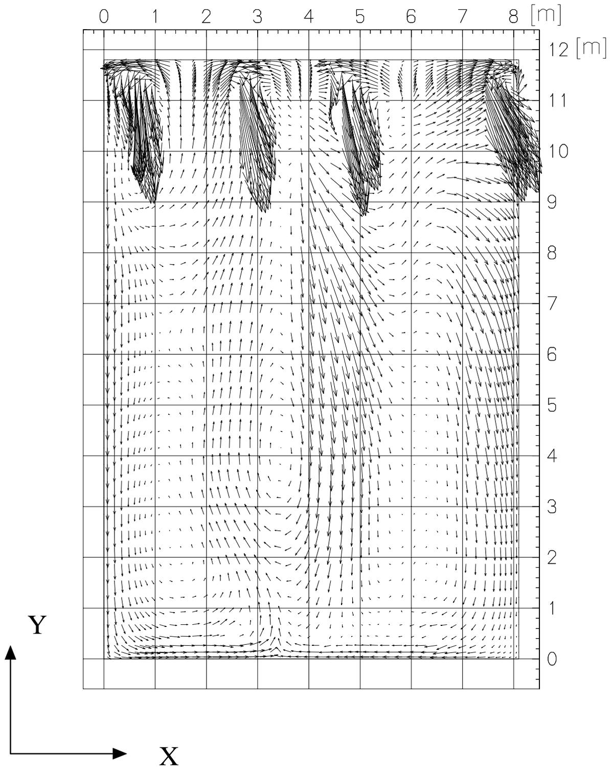
Fig. 4 Velocity vectors at a height of  $z = 2.0$  [m]
