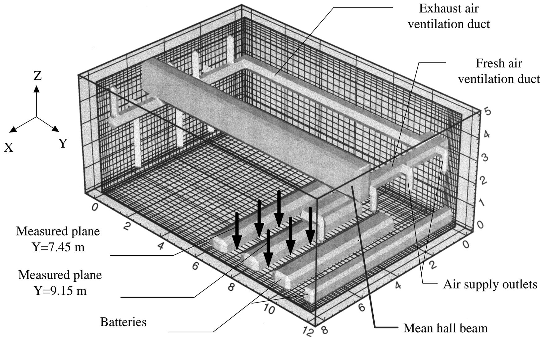
Fig. 1 The layout of the room with the numerical mesh
