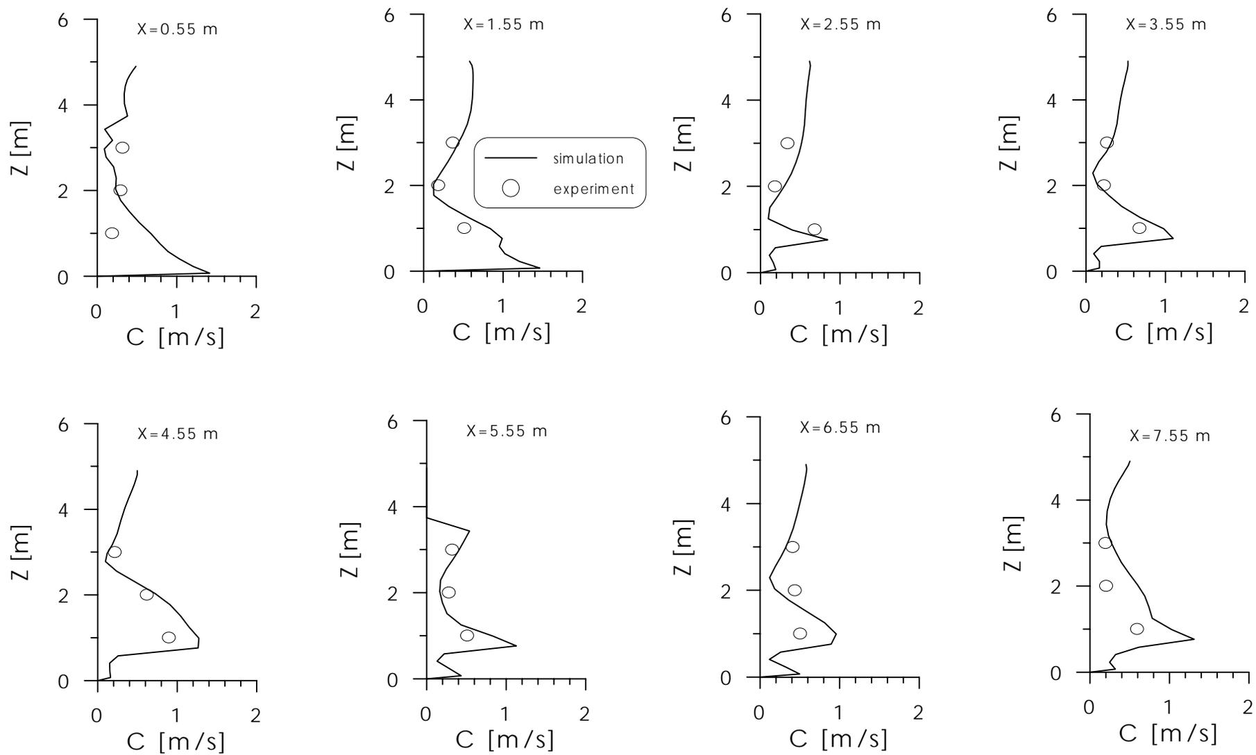
Fig. 2 The size of the velocity vectors at different locations in the plane  $Y=7.45$  m
