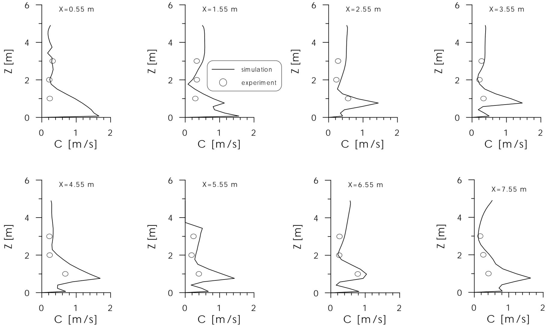
Fig. 3 The size of the velocity vectors at different locations in the plane  $Y=9.15$  m
