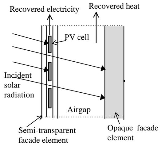
Figure 1: PV-integrated Facade
