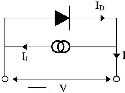
Figure 3: Equivalent Circuit for a p-n Junction with Light
