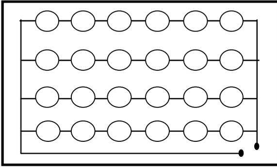
Figure 2: Example PV Panel (n=6, m=4)
