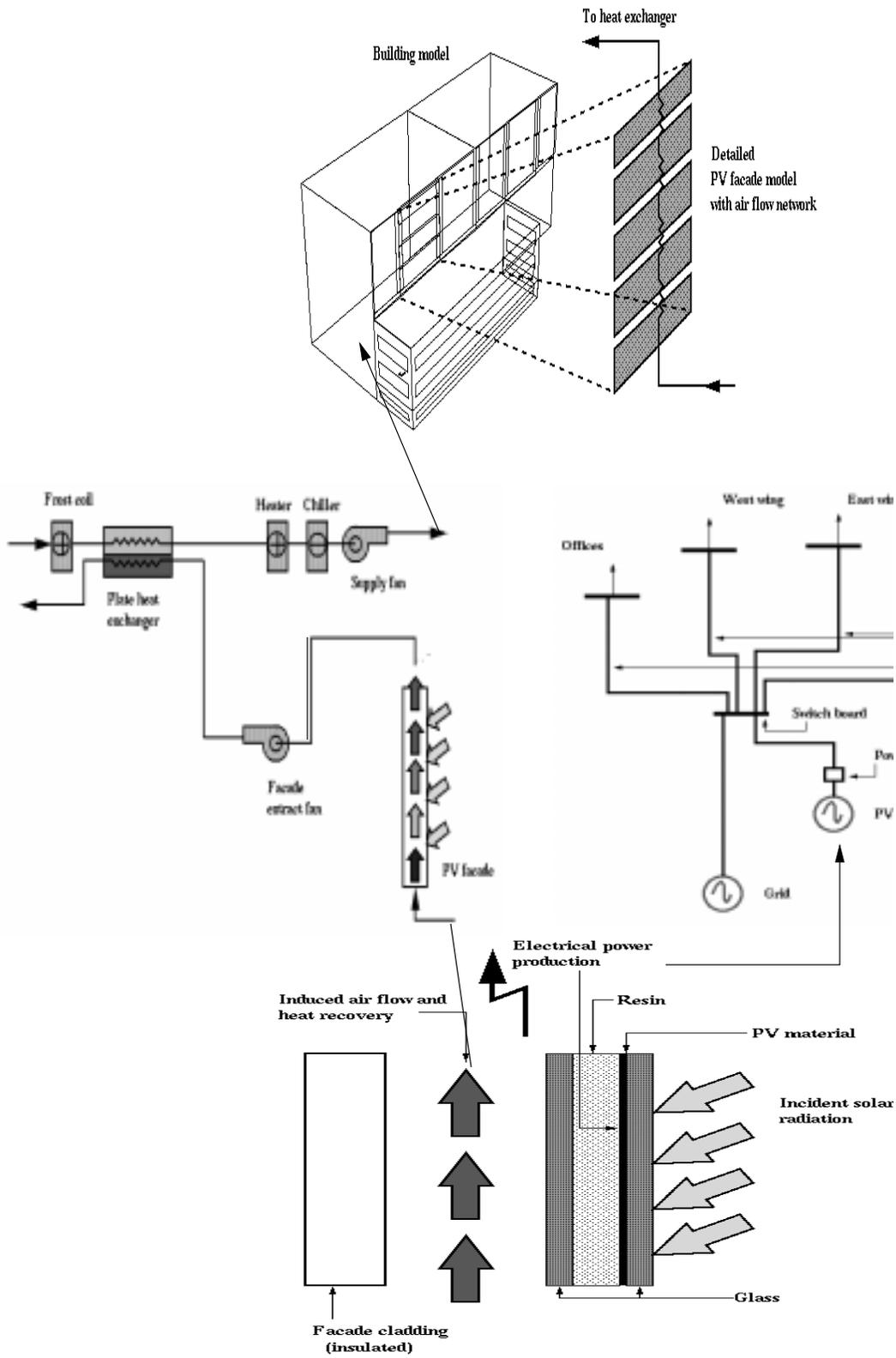
Figure 4: ESP-r's integrated PV model
