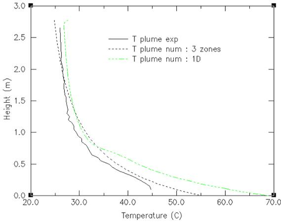
**Figure 8 : plume temperature in case 1**
