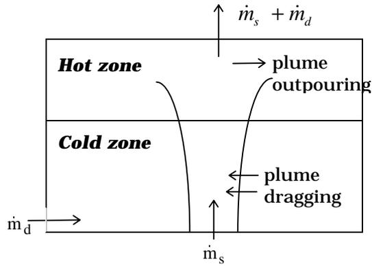
Figure 1 : principle of a displacement ventilation system
