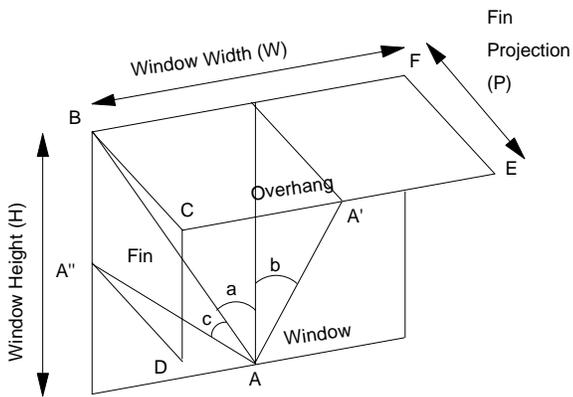
Figure 3: Example solar shading device that consists of an overhang and a right vertical fin.
