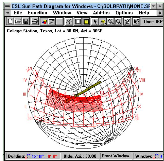
FIGURE 2: Sunpath diagram and rotated shading mask protractor. In this view the shading mask protractor has been added to the sunpath previously shown in Figure 1 and rotated 30 degrees east of south. The window frame for a window that is 4 ft in width by 3 ft in height is also shown.
