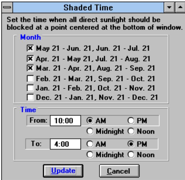
FIGURE 8: Solar Target Time. This figure shows the data input screen for the time of day, and time of year that shading is to be provided for Figure 6.
