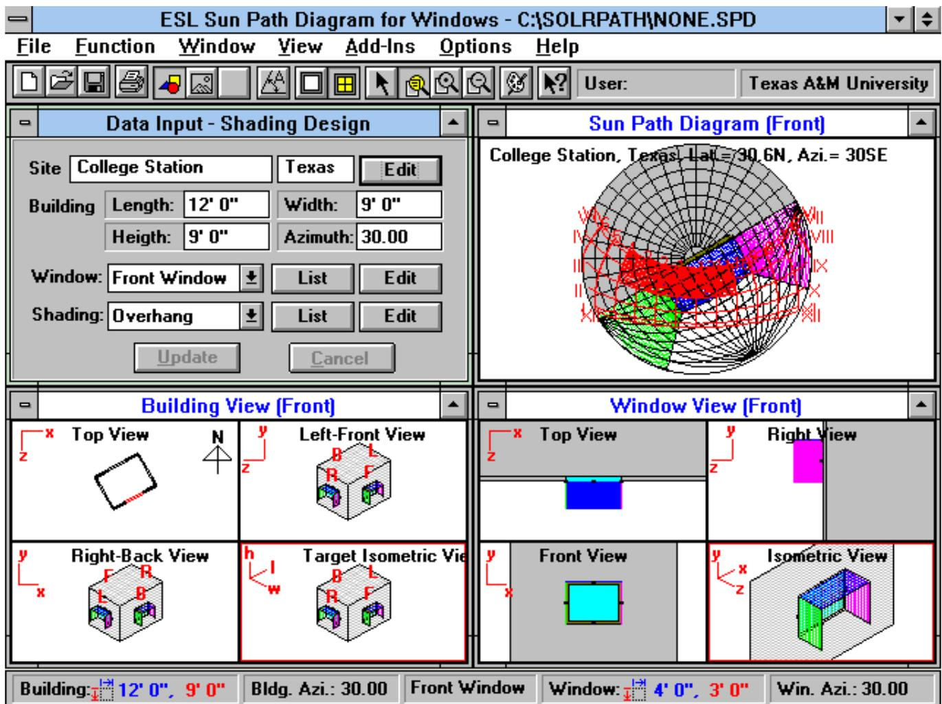
FIGURE 6: Opening screen for the MS Windows solar shading analysis program. This figure shows the opening screen for the sunpath shading analysis program. All data entry is made in the "data input" screen. Modifications to the shading devices are shown on the various views of the building and the effect of the shading is shown on the combined sunpath diagram and shading mask protractor.
