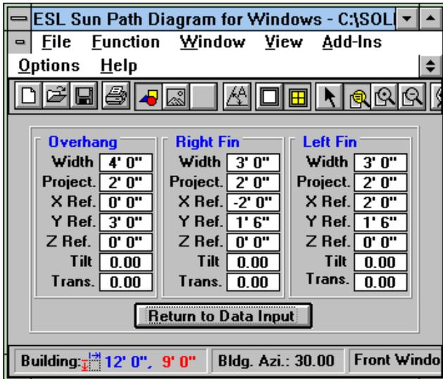
FIGURE 7: Data Input Summary Screen. This figure shows the data input screen where all pertinent data for the currently displayed facade are shown. The data shown represent the dimensions of the horizontal shade and left and right fins shown in Figure 6.
