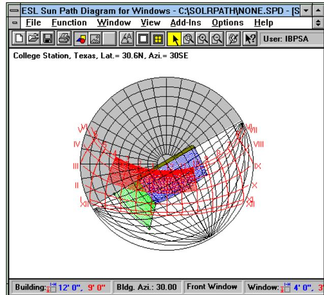
Figure 5: Sunpath diagram and shading from overhead shade and 2 ft by 2 ft right fin. This view shows the combined shading from the previously described overhead shade and a 2 ft. by 2 ft. fin placed directly below the overhead on the right side of the window (as the viewer faces out).
