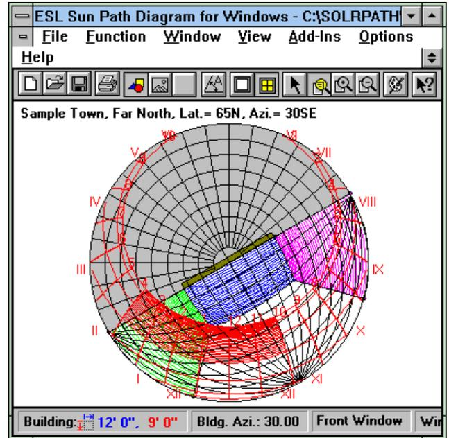
FIGURE 9: Sunpath Diagram and Shading Mask Protractor for 65 Degrees North Latitude. This combined diagram shows the sunpath diagram and shading mask protractor for a vertical surface facing 30 degrees east of south.
