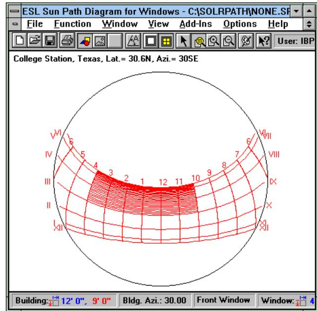
FIGURE 1: Sunpath diagram for a northern latitude of 30.6 degrees with a target shading time of 10:00 a.m. to 4:00 p.m. indicated from March through September.
