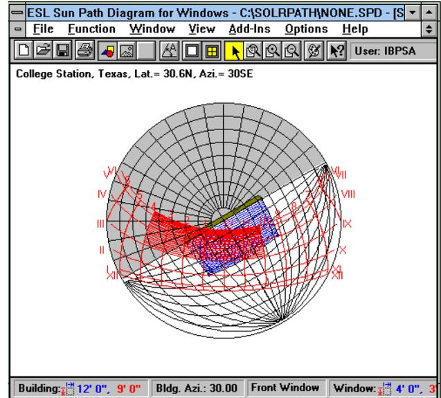
Figure 4: View of sunpath and shading from 2 ft. overhang. This sunpath diagram contains the previously described sunpath and the shading for a 2 ft. overhang that projects directly out from the top of the window.
