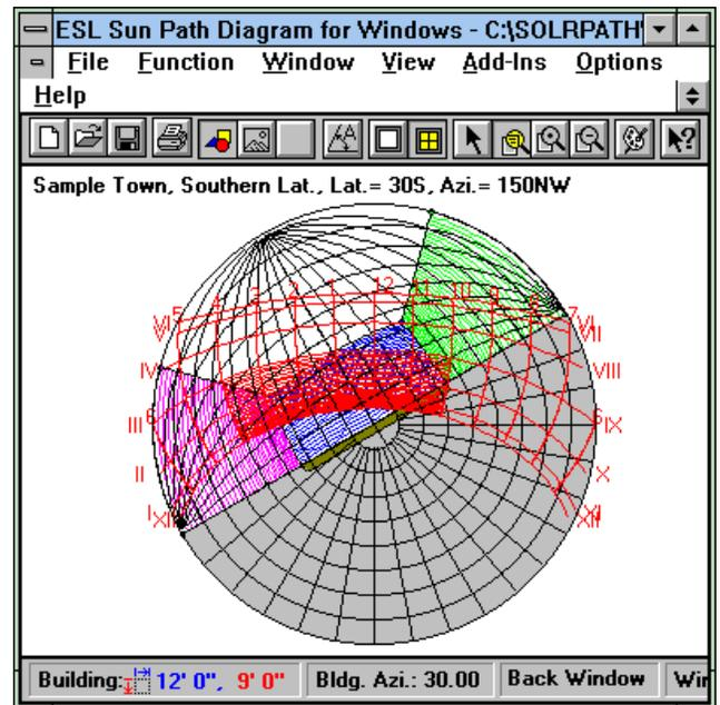
FIGURE 10: Sunpath Diagram and Shading Mask Protractor for 30 Degree South Latitude. This combined diagram shows the sunpath diagram and shading mask protractor for a vertical surface facing 30 degrees west of north for a period from September through March.
