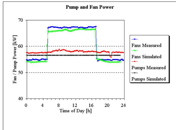
Figure 7: Fan and pump power for second system.
