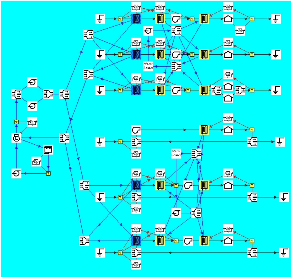
Figure 2 : Schematic of second HVAC system
