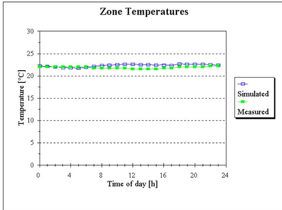
**Figure 9: Zone temperature for a zone in first system.**
