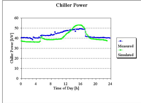
Figure 6: Chiller power for second system
