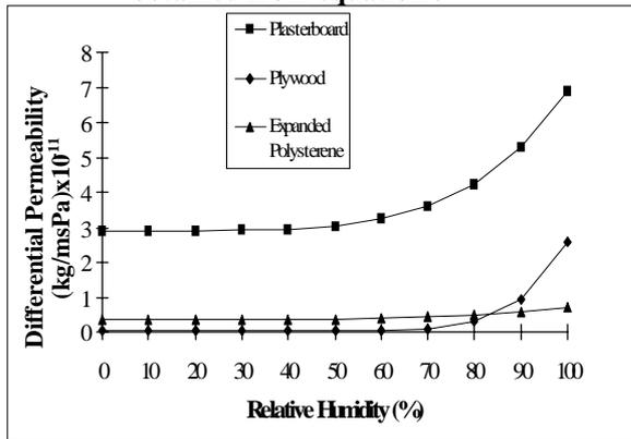
The differential permeability curves for equation type 4 (Figure 3) clearly exhibit a different shape from that produced by equations 1 and 3.
