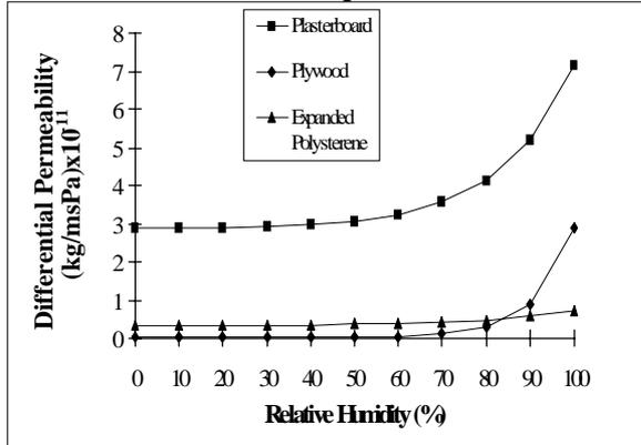
**Figure 2 Differential permeability curves obtained from equation 3**
