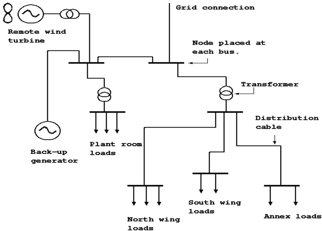
Figure 3: An ESP-r power flow network.
