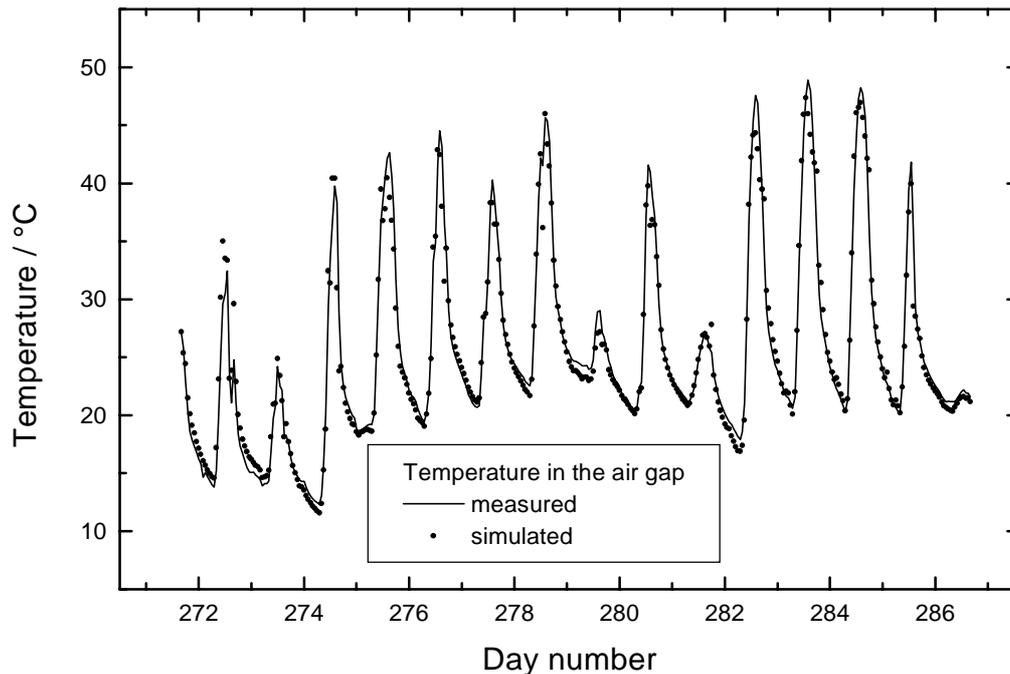
Fig. 4: Measured and simulated temperature in the air gap
