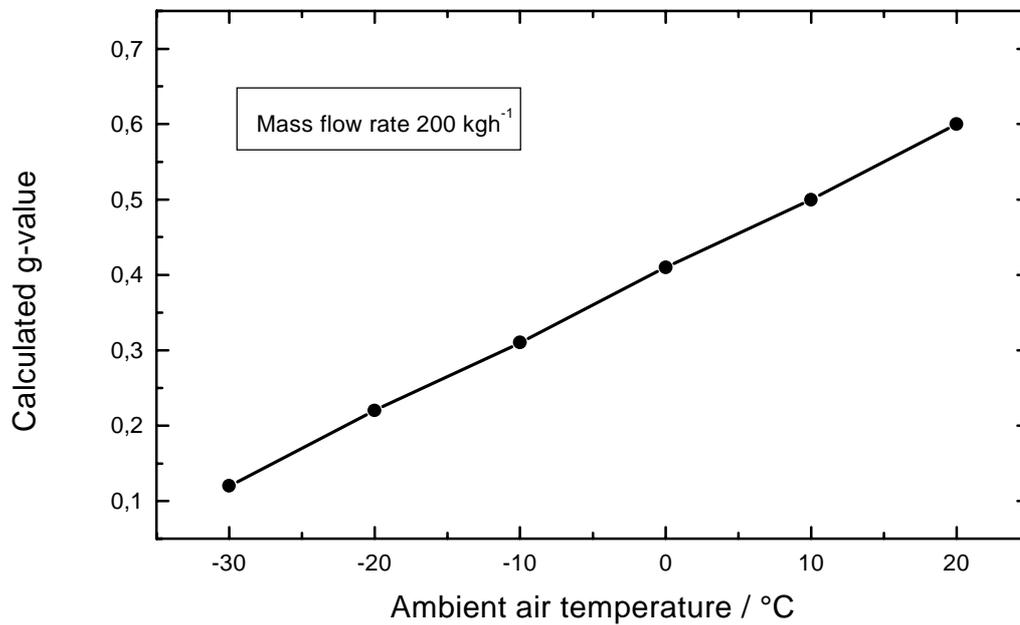
*Fig. 7:* Solar transmittance in dependence on the ambient air temperature
