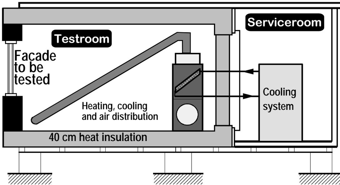
Fig. 2: Cross section of a PASSYS test cell
