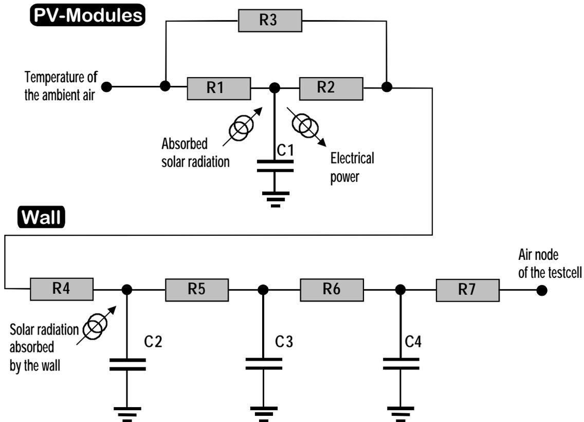
Fig. 3: RC network as thermal model for the PV facade
