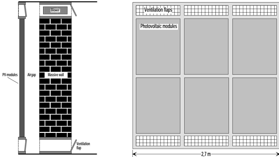
*Fig. 1:* The photovoltaic facade
