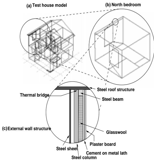
Figure 3: ESP-r model of test house.
