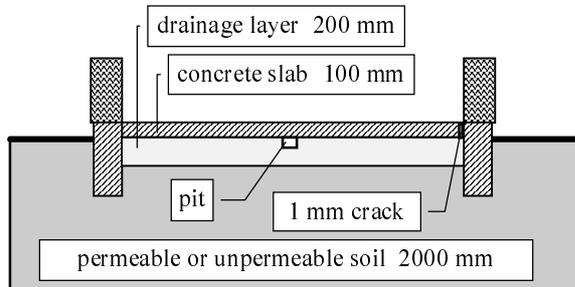
**Fig. 1a** Cross section of the theoretical model
