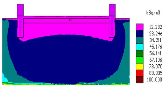
**Fig. 6b Results for soil pressurization system (+ 50 Pa) in the permeable soil under slab with drainage layer and no crack - the radon concentration field**
