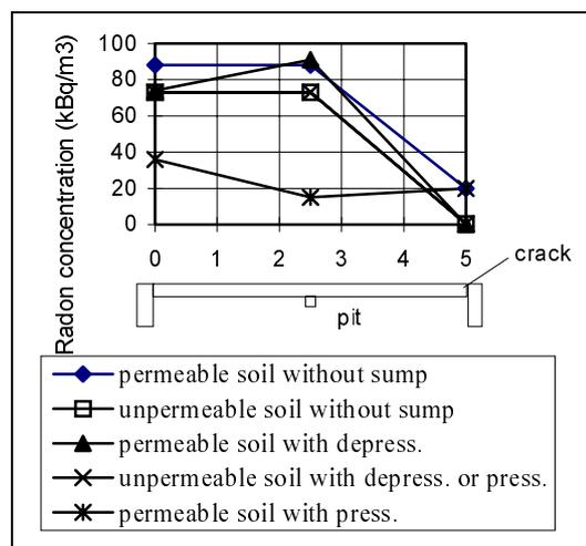
**Fig. 4b Radon concentration in the soil immediately beneath the untight concrete slab**
