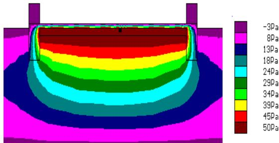
**Fig. 6a Results for soil pressurization system (+ 50 Pa) in the permeable soil under slab with drainage layer and no crack - the pressure field**
