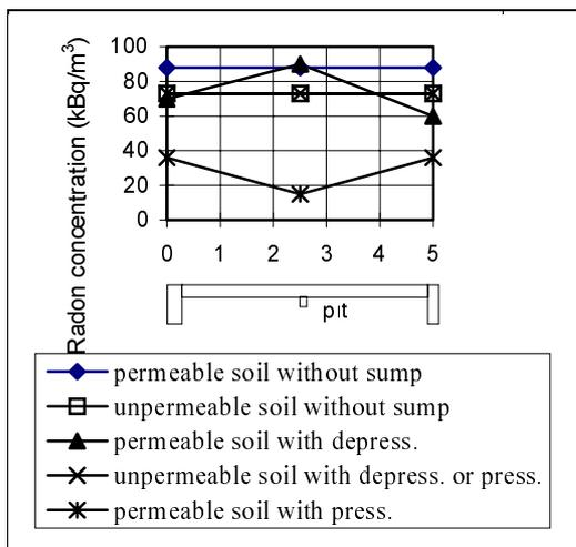
**Fig. 4a Radon concentration in the soil immediately beneath the tight concrete slab**
