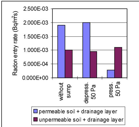
**Fig. 2a Radon entry rate in case of tight concrete slab and drainage layer**
