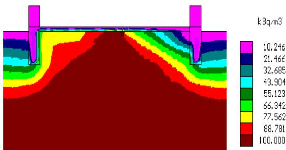
**Fig. 5b Results for soil depressurization system (- 50 Pa) in the permeable soil under slab with crack and no drainage layer - the radon concentration field**
