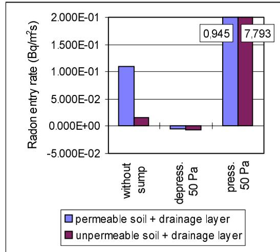
**Fig. 2b Radon entry rate in case of untight concrete slab and drainage layer**
