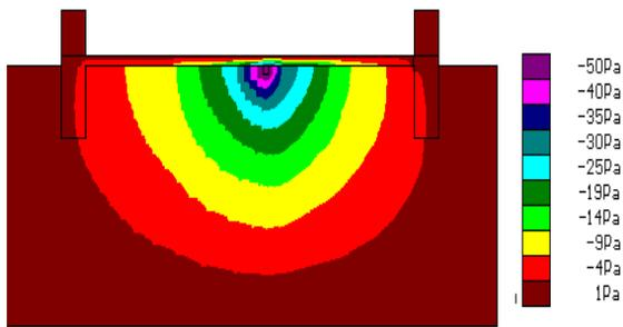
**Fig. 5a Results for soil depressurization system (- 50 Pa) in the permeable soil under slab with crack and no drainage layer - the pressure field**
