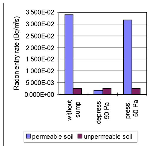
**Fig. 3b Radon entry rate in case of untight concrete slab and no drainage layer**
