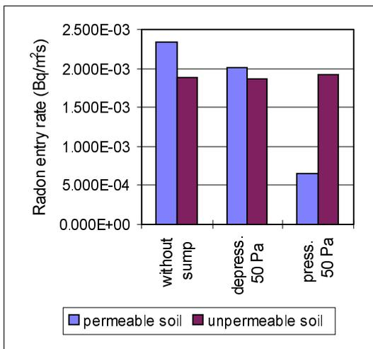
**Fig. 3a Radon entry rate in case of tight concrete slab and no drainage layer**
